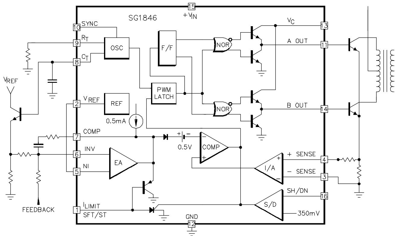
FIGURE 25 - PUSH/PULL CONVERTER WITH SLOPE COMPENSATION
