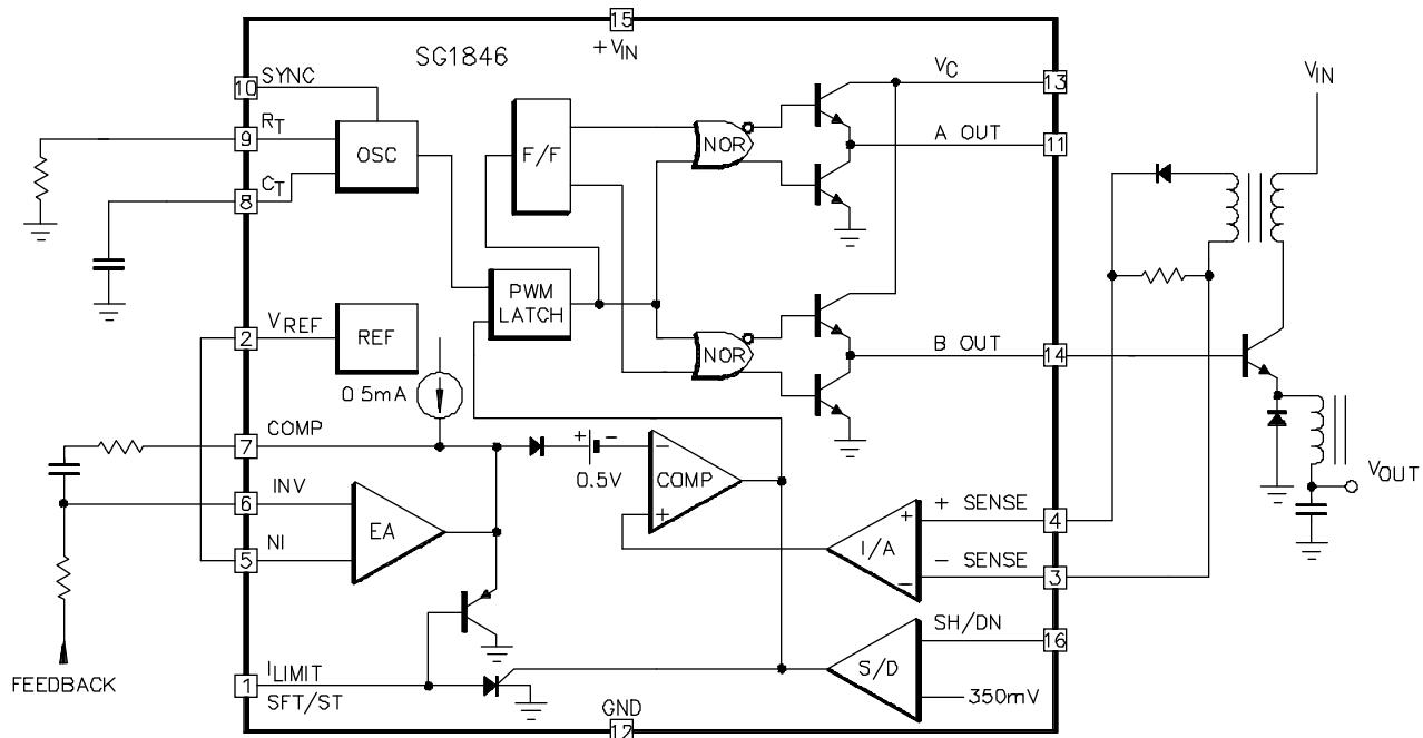
FIGURE 24 - BUCK CONVERTER WITH CURRENT SENSE WINDING
