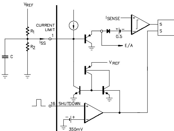
FIGURE 27 - SOFT START AND SHUTDOWN/RESTART FUNCTIONS
