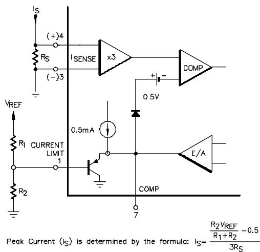
FIGURE 26 - PULSE BY PULSE CURRENT LIMITING
