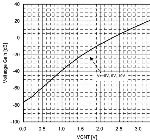
Voltage Gain vs. Control Voltage (Frequency)
