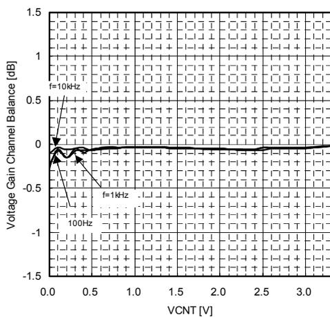
Voltage Gain Channel Balance vs. Control Voltage (Ambient Temperature)
