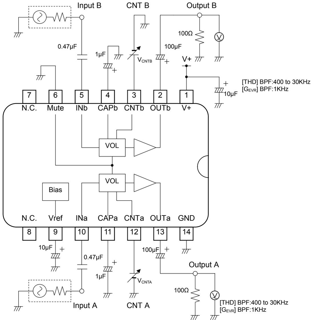
$$\text{Volume Range : } GEVR = 20 \log \frac{V_{o \max}}{V_{o \min}}$$
