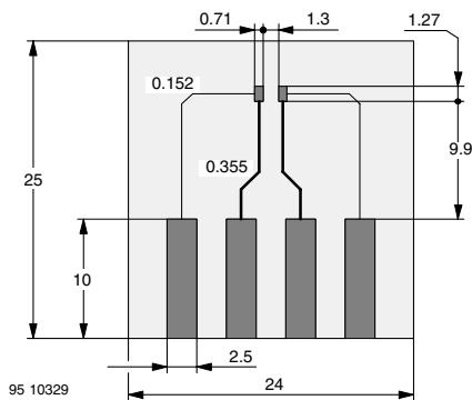
Figure 5. Board for  $R_{thJA}$  definition (in mm)
