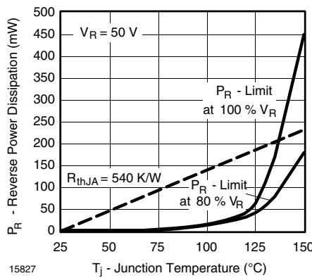
Figure 1. Max. Reverse Power Dissipation vs. Junction Temperature
