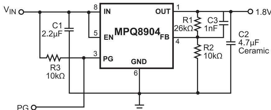
**Figure 2: Typical Application Circuit**
