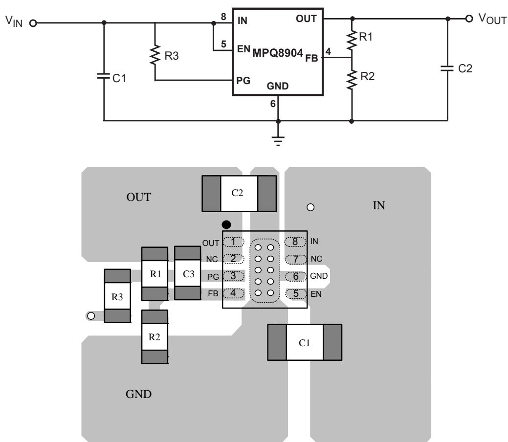
Figure 3: PCB Layout, Top Layer
