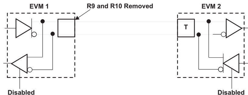
Figure 5. Point-to-Point Simplex Circuit
