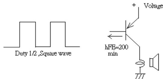
The base current,  $I_b$ , should be high enough so that it saturates the collector current of the transistor with the CB load.
