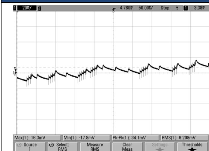
Ripple and Noise @25°C (Vin = 110V, Vout = nom., Iout = 0, Cload = 0, ScopeBW = 20MHz)
