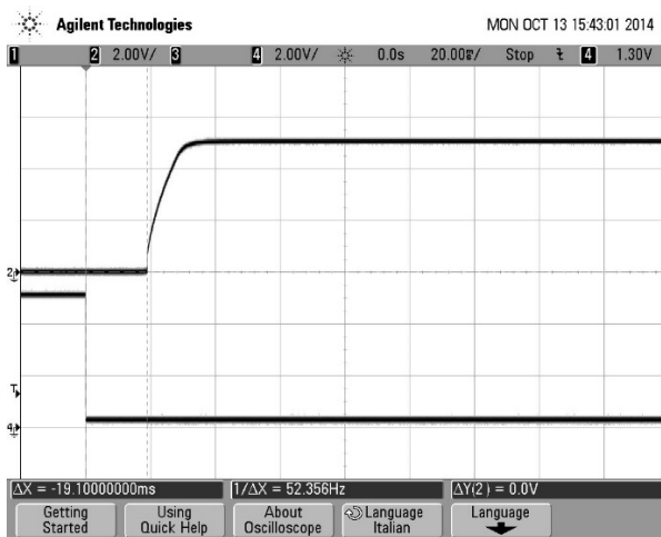
Turn-on transient at zero load current (20 mS/div, Top Trace: Vout, 2V/div; Bottom Trace: ON/OFF, 2V/div)
