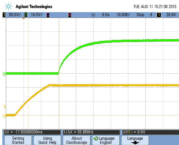
Turn-on transient at full load current (10 mS/div, Top Trace: Vout, 10V/div; Bottom Trace: Vin, 50V/div)
