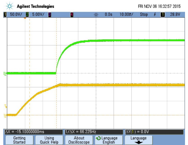
Turn-on transient at full load current (10 mS/div, Top Trace: Vout, 5V/div; Bottom Trace: Vin, 50V/div)
