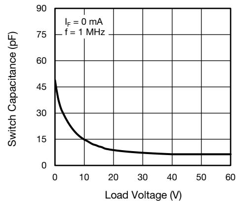
Fig. 10 - Switch Capacitance vs. Load Voltage
