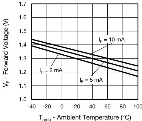
Fig. 6 - Forward Voltage vs. Ambient Temperature
