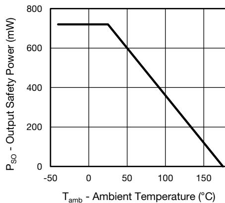
Fig. 3 - Output Safety Power vs. Ambient Temperature
