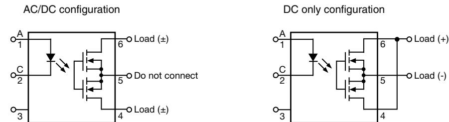
Fig. 1 - Pin Configuration
