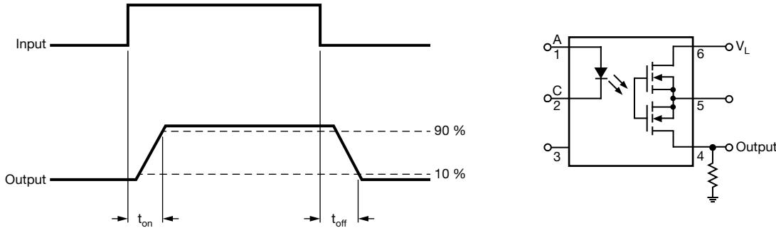
Fig. 2 - Timing Schematic
