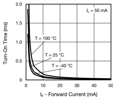
Fig. 12 - Turn-On Time vs. Forward Current
