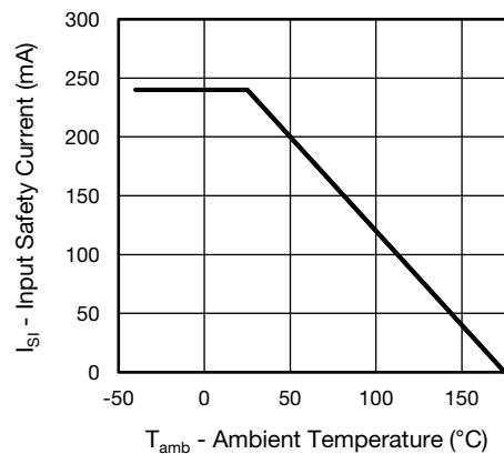
Fig. 4 - Input Safety Current vs. Ambient Temperature
