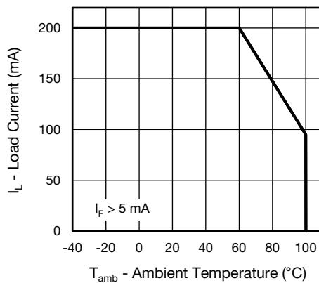
Fig. 5 - Load Current vs. Ambient Temperature
