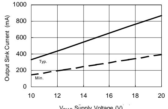
**Figure 20B. Output Sink Current vs. Supply Voltage**
