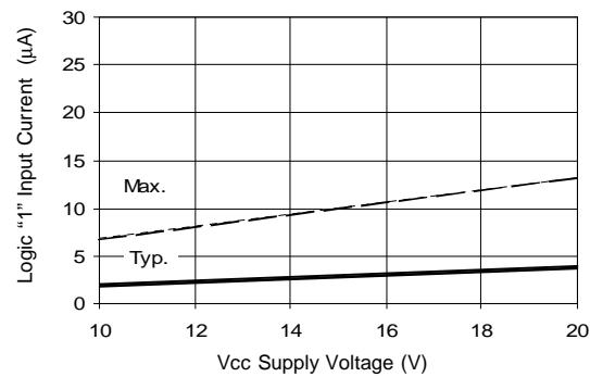
**Figure 16B. Logic "1" Input Current vs. Voltage**
