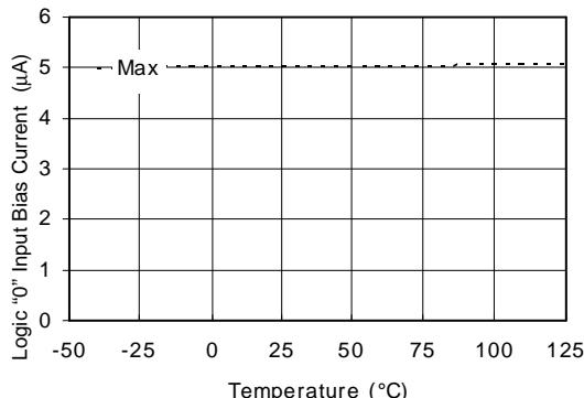
**Figure 17A. Logic "0" Input Bias Current vs. Temperature**
