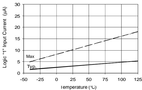
**Figure 16A. Logic "1" Input Current vs. Temperature**
