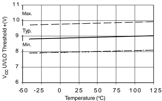
**Figure 18A. V<sub>CC</sub> Undervoltage Threshold(+) vs. Temperature**
