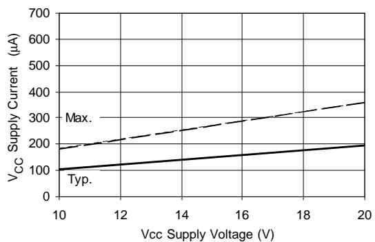
**Figure 15B. V<sub>CC</sub> Supply Current vs. Voltage**
