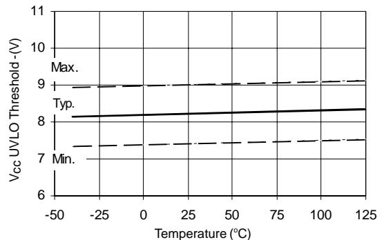
**Figure 18B. V<sub>CC</sub> Undervoltage Threshold (-) vs. Temperature**
