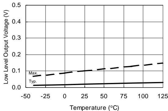
**Figure 12A. Low Level Output Voltage vs. Temperature**
