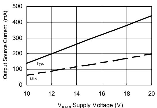
**Figure 19B. Output Source Current vs. Supply Voltage**
