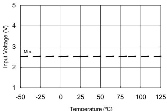
**Figure 9A.** Logic "1" Input Voltage
