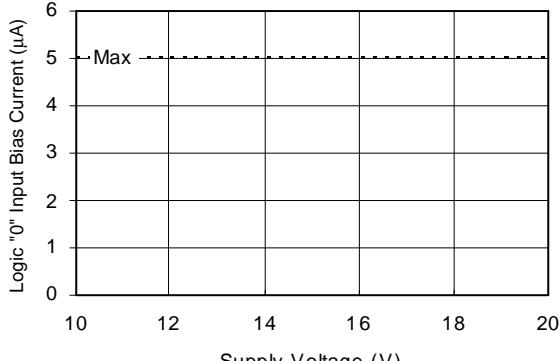
**Figure 17B. Logic "0" Input Bias Current vs. Voltage**
