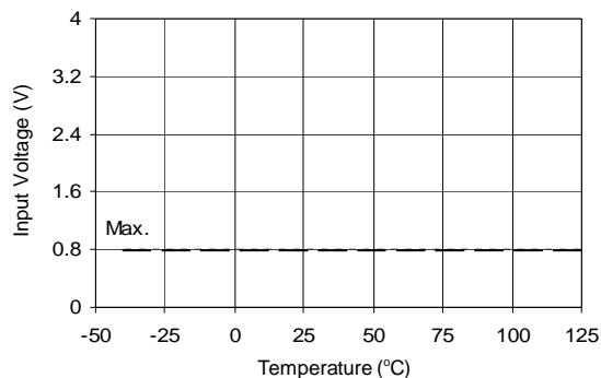
**Figure 10A.** Logic "0"(HIN) & Logic "1" (LIN)
