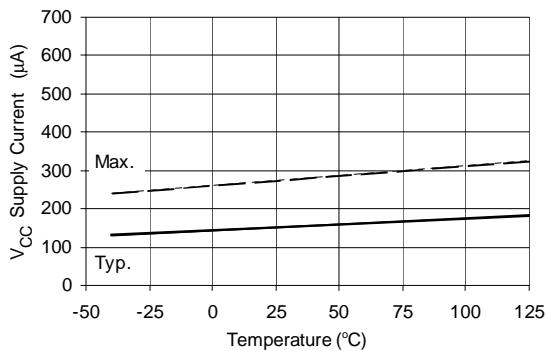
**Figure 15A. V<sub>CC</sub> Supply Current vs. Temperature**
