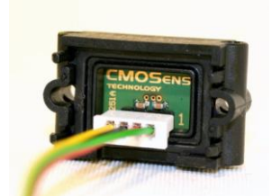
Figure 2 Pin assignment of SDP6xx on PCB top view from left to right. Connect cable such that yellow cable is connected to data, black (GND), red (Vdd) and green (clock).
