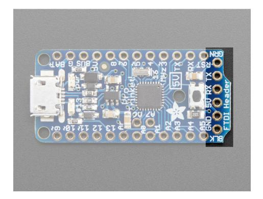
The bootloader on Pro Trinket is **dual USB & FTDI** "optiboot" so you can use either the USB port or the FTDI breakout to upload. However, only the FTDI port allows you to use Serial debugging. So it's a bit of a tradeoff - USB is inexpensive, built-in but requires a button press to start & there's no debugging, FTDI requires an extra cable but has auto-reset and debug console.
