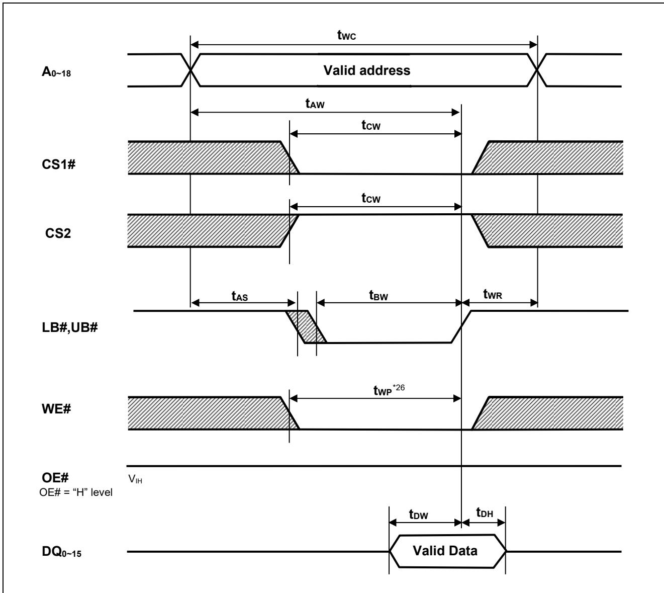
Note 26.  $t_{WP}$  is the interval between write start and write end.
