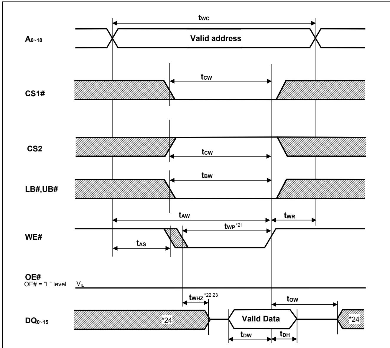
Note 21. t<sub>WP</sub> is the interval between write start and write end.
