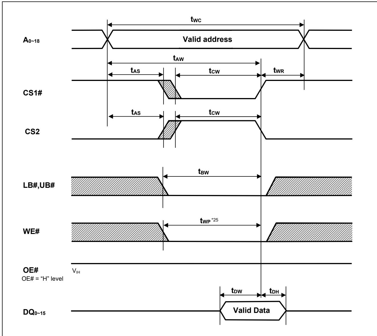
Note 25.  $t_{WP}$  is the interval between write start and write end.
