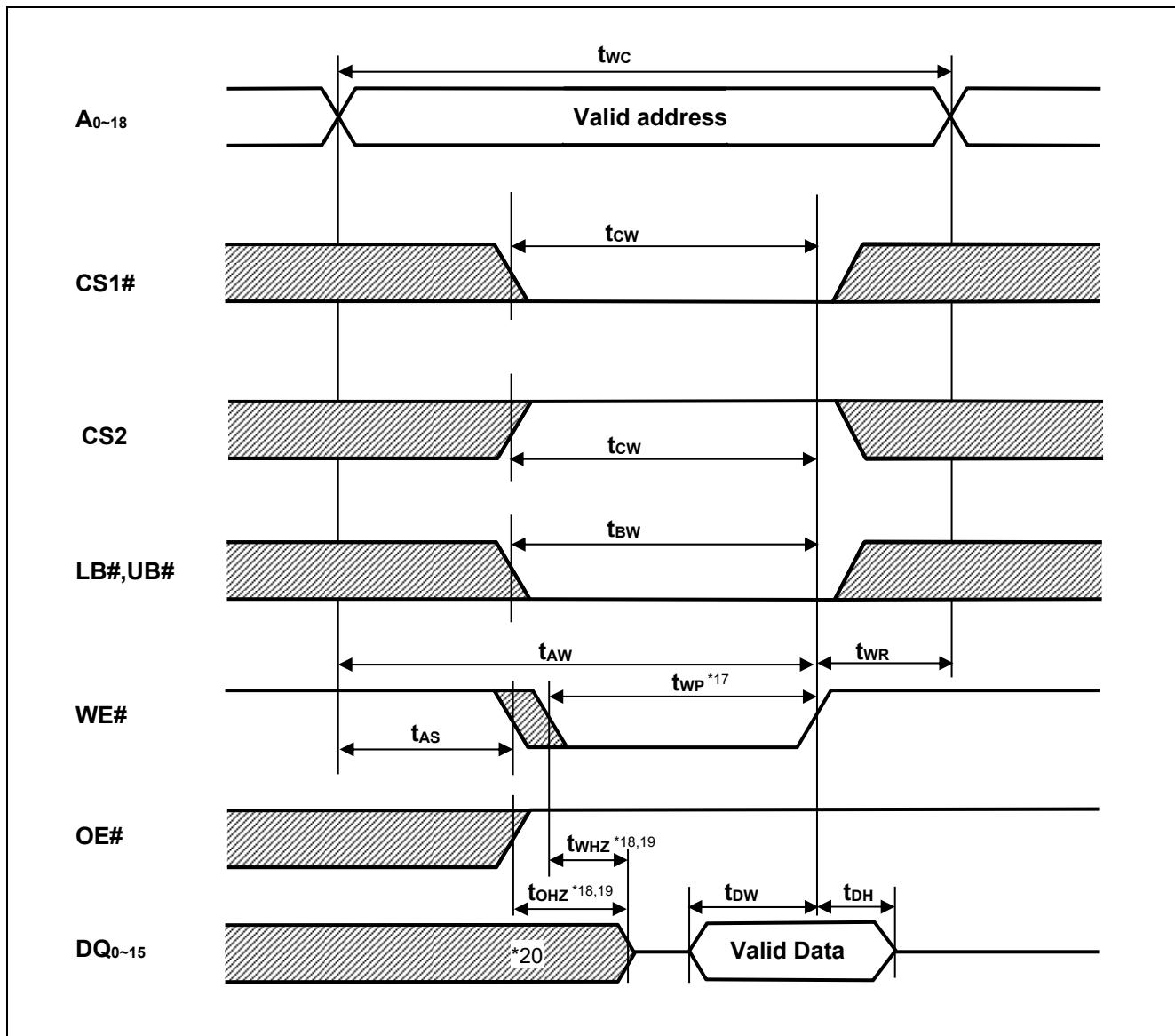
Note 17. t<sub>WP</sub> is the interval between write start and write end.
