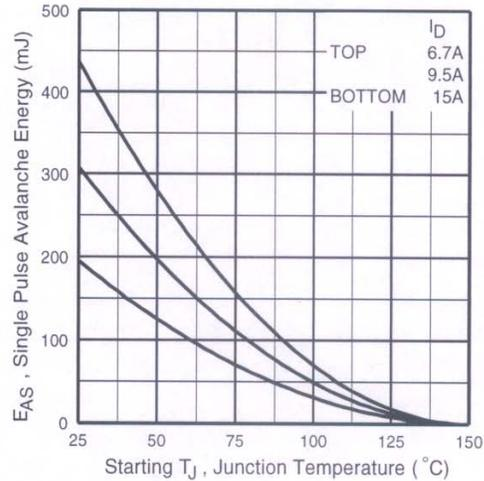
**Fig 14c.** Maximum Avalanche Energy Vs. Drain Current
