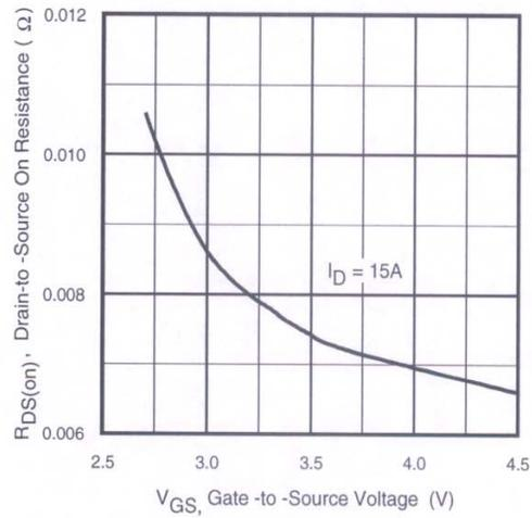
**Fig 13.** On-Resistance Vs. Gate Voltage
