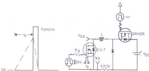
**Fig 14a&b.** Unclamped Inductive Test circuit and Waveforms
