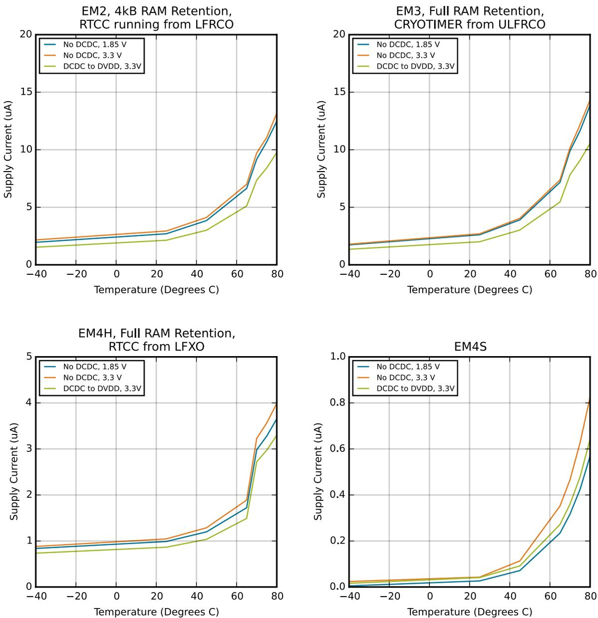
Figure 4.5. EM2, EM3, EM4H and EM4S Typical Supply Current
