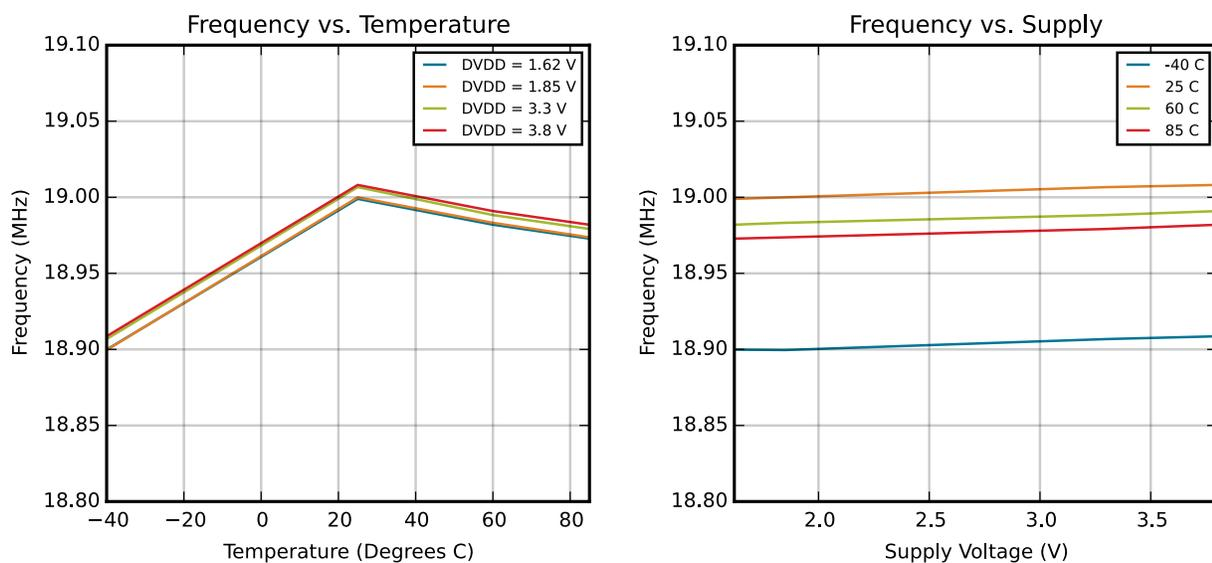
**Figure 4.11. HFRCO and AUXHFRCO Typical Performance at 19 MHz**
