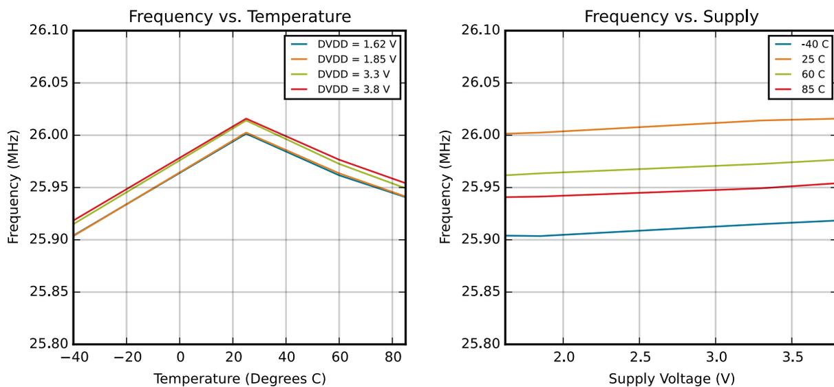
**Figure 4.10. HFRCO and AUXHFRCO Typical Performance at 26 MHz**
