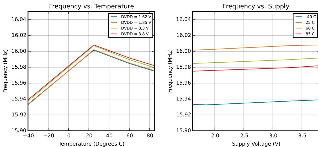
**Figure 4.12. HFRCO and AUXHFRCO Typical Performance at 16 MHz**
