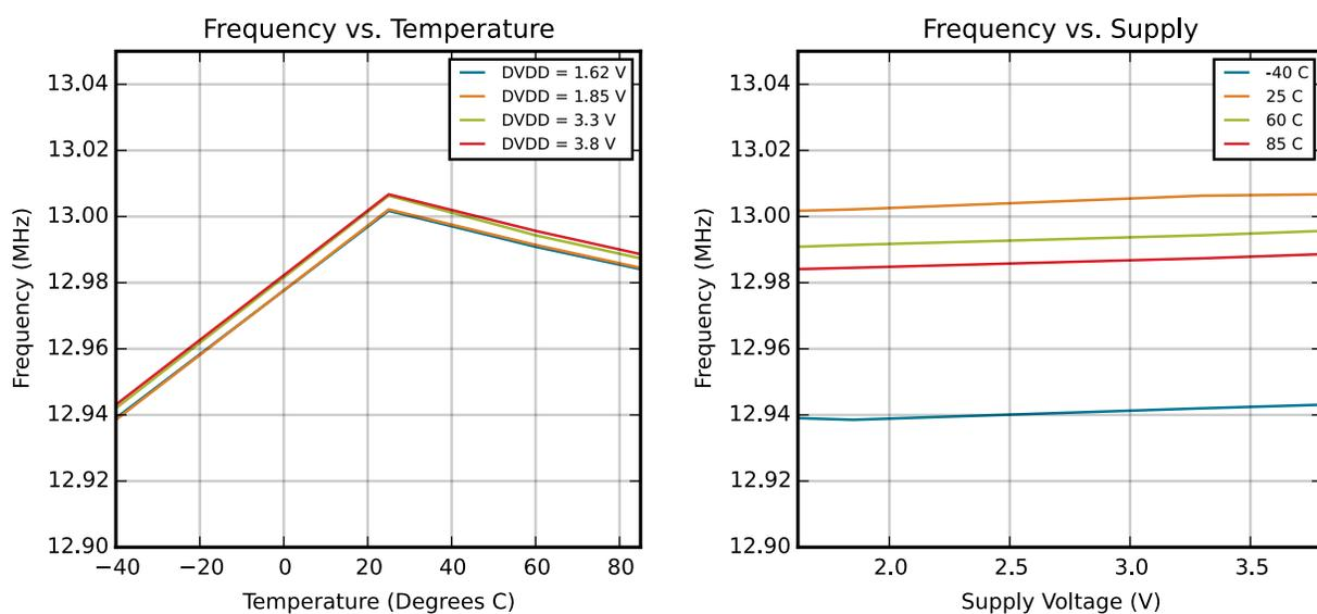
**Figure 4.13. HFRCO and AUXHFRCO Typical Performance at 13 MHz**
