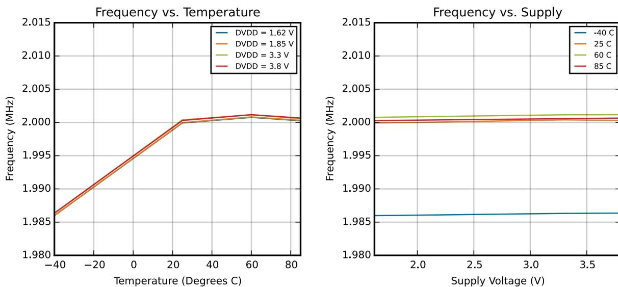
Figure 4.16. HFRCO and AUXHFRCO Typical Performance at 2 MHz
