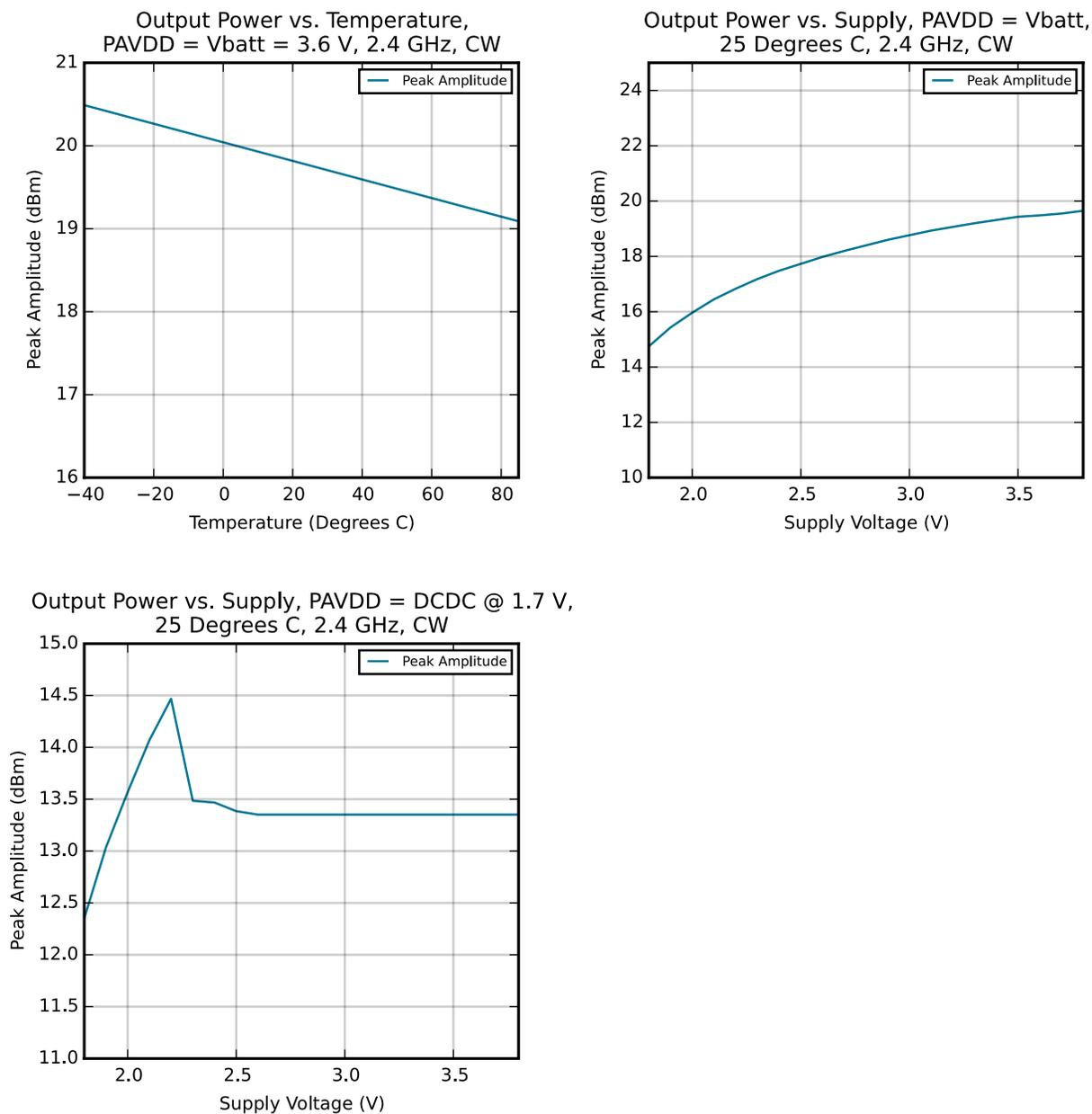
Figure 4.20. 2.4 GHz RF Transmitter Output Power
