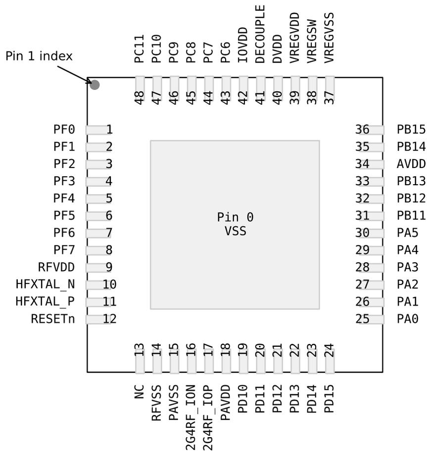
Figure 6.1. EFR32MG1 QFN48 2.4 GHz Pinout
