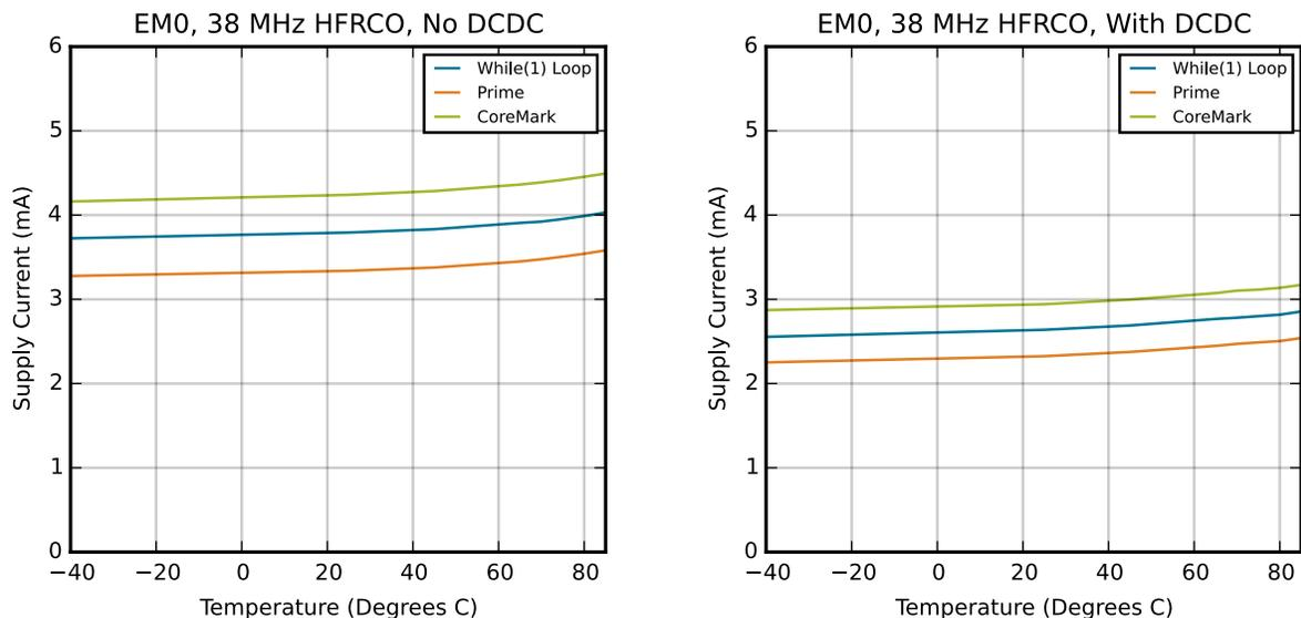
Figure 4.3. EM0 Active Mode Typical Supply Current
