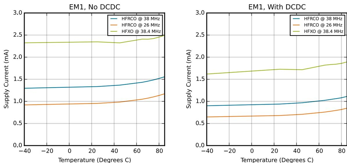
Figure 4.4. EM1 Sleep Mode Typical Supply Current
