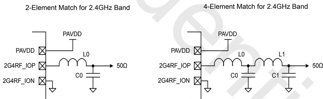
Figure 5.4. Typical 2.4 GHz RF impedance-matching network circuits
