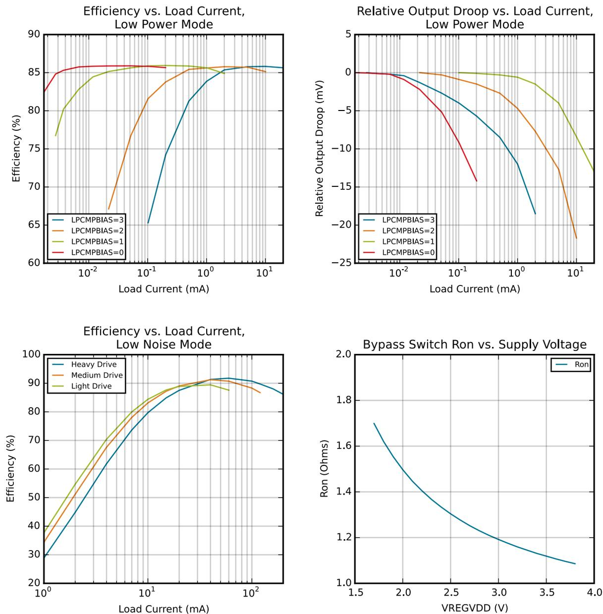
Figure 4.6. DC-DC Converter Typical Performance Characteristics
