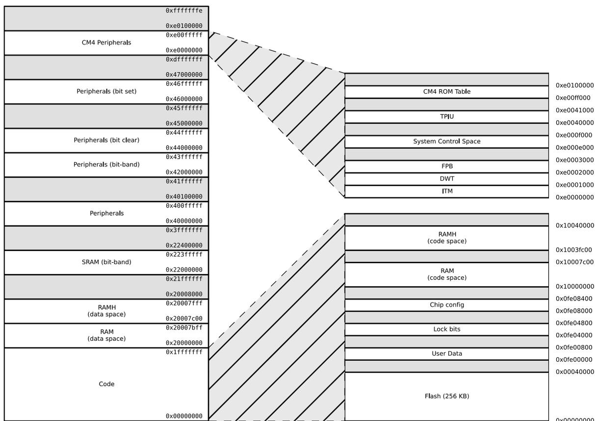
Figure 3.2. EFR32MG1 Memory Map — Core Peripherals and Code Space
