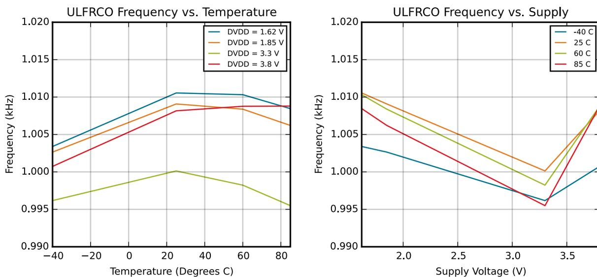
Figure 4.19. ULFRCO Typical Performance at 1 kHz
