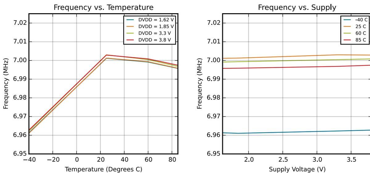
Figure 4.14. HFRCO and AUXHFRCO Typical Performance at 7 MHz
