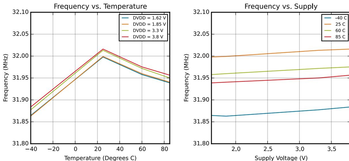
Figure 4.9. HFRCO and AUXHFRCO Typical Performance at 32 MHz
