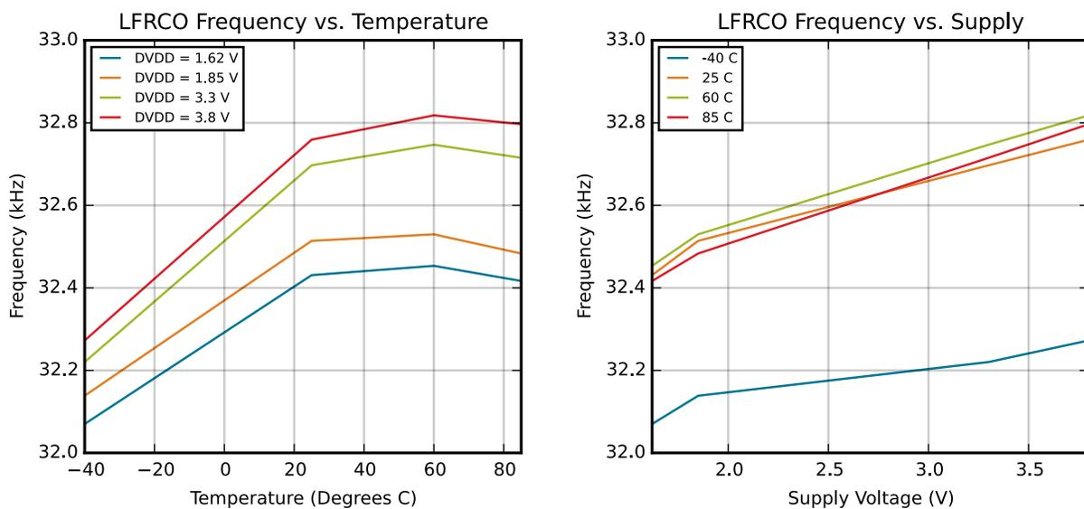
Figure 4.18. LFRCO Typical Performance at 32.768 kHz
