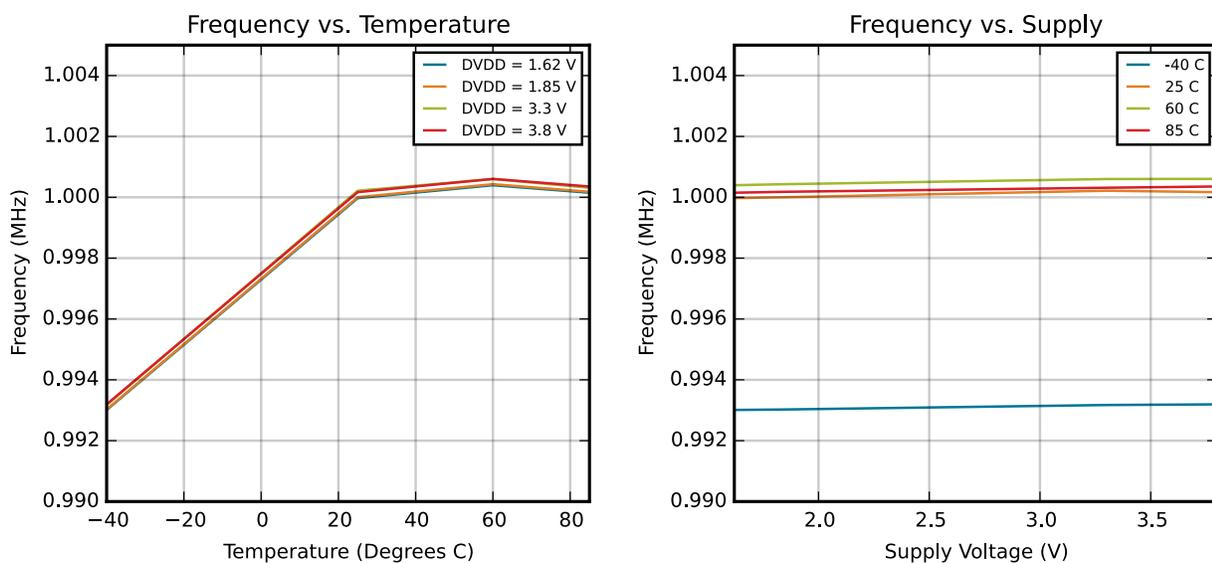
Figure 4.17. HFRCO and AUXHFRCO Typical Performance at 1 MHz
