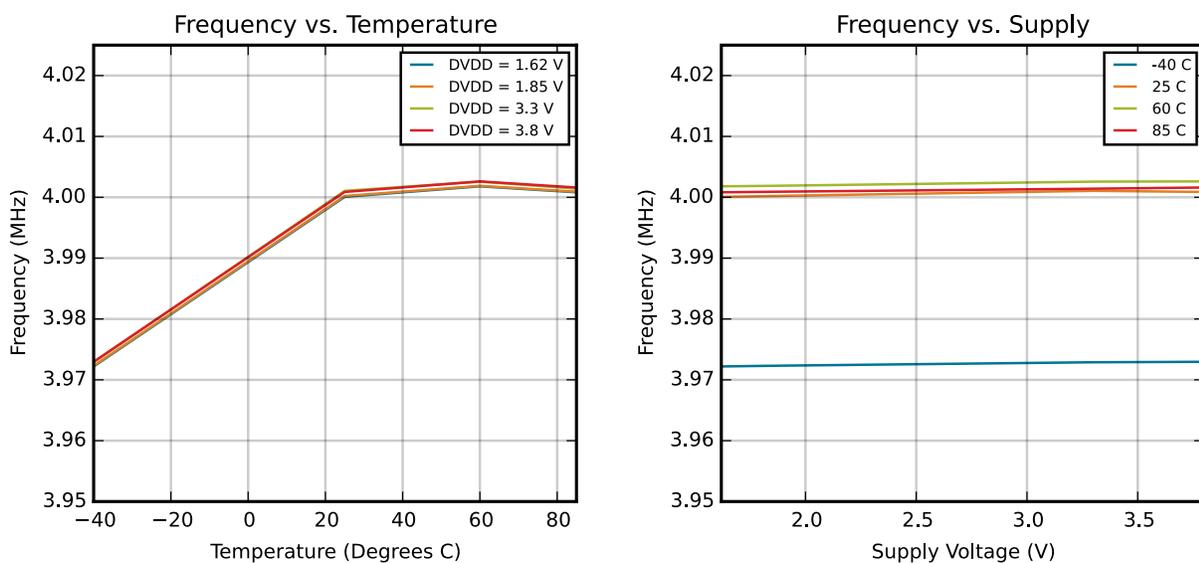
Figure 4.15. HFRCO and AUXHFRCO Typical Performance at 4 MHz
