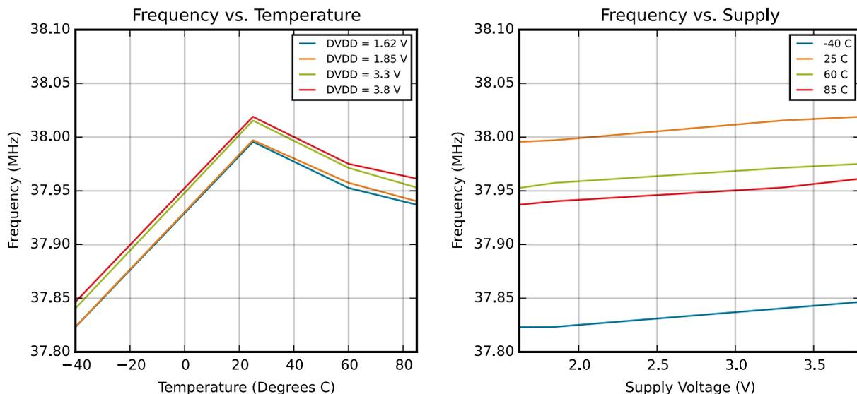
Figure 4.8. HFRCO and AUXHFRCO Typical Performance at 38 MHz
