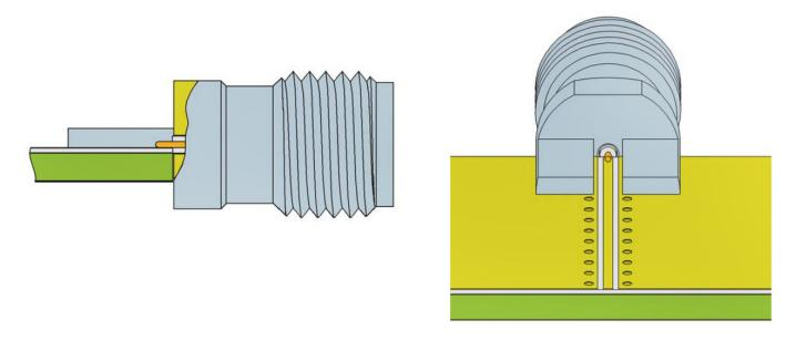
Figure 1 - End Launch Connector Shown Attached to the GCPW Transmission Line
