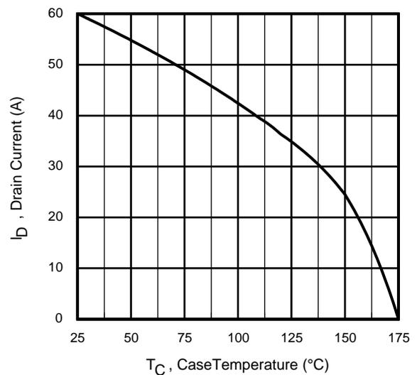
Fig 2. Maximum Drain Current vs. Case Temperature
