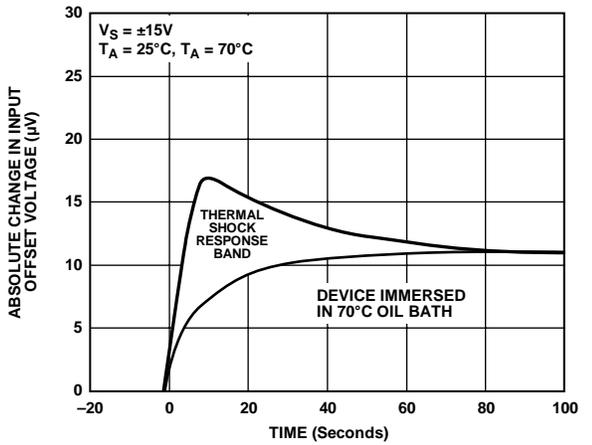
Figure 4. Offset Voltage Change due to Thermal Shock
