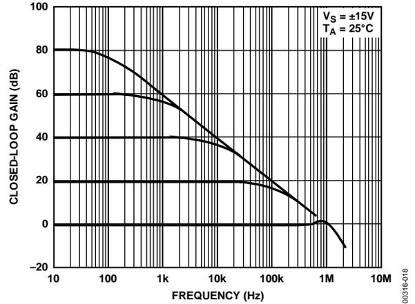
Figure 18. Closed-Loop Frequency Response for Various Gain Configurations
