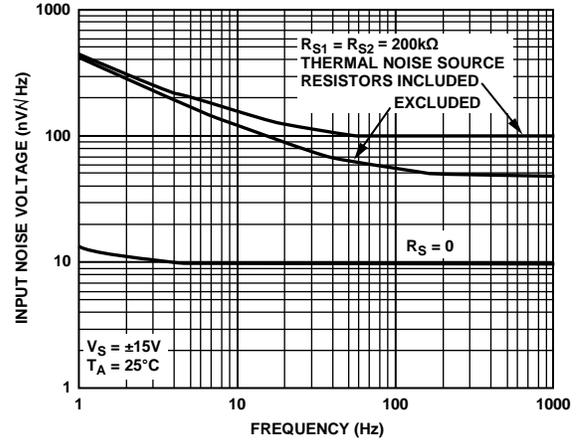
Figure 12. Total Input Noise Voltage vs. Frequency
