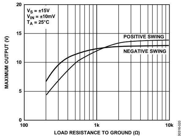
Figure 20. Maximum Output Voltage vs. Load Resistance
