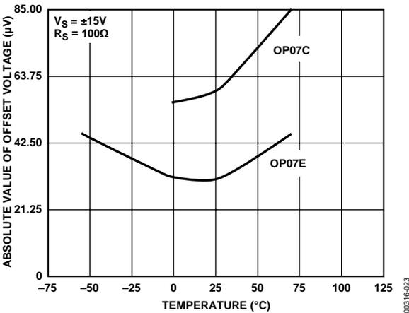
Figure 23. Untrimmed Offset Voltage vs. Temperature
