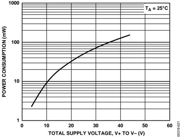
Figure 21. Power Consumption vs. Power Supply
