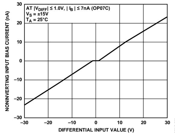
Figure 8. Input Bias Current vs. Differential Input Voltage
