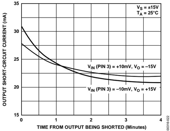
Figure 22. Output Short-Circuit Current vs. Time
