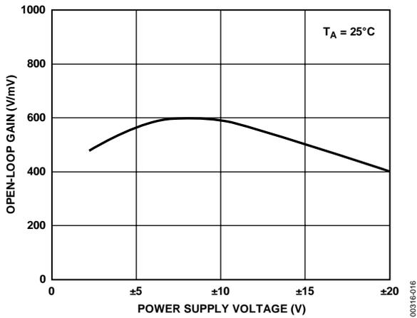
Figure 16. Open-Loop Gain vs. Power Supply Voltage
