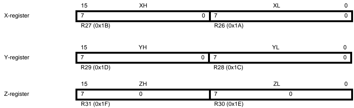
Figure 6-5. The X-, Y-, and Z-registers
