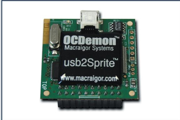
The usb<sup>2</sup>Sprite is a self-powered, cable-less, miniaturized (2.25 in<sup>2</sup>) version of our usb<sup>2</sup>Demon that plugs directly into a board's JTAG/BDM header providing "built-in" debug connectivity. To the user the usb<sup>2</sup>Sprite looks like a USB mini connector sitting on top of the board's JTAG/BDM header. Problems caused by customer installation errors, JTAG cable noise, parallel port incompatibility, and the need for an external power supply are eliminated.
