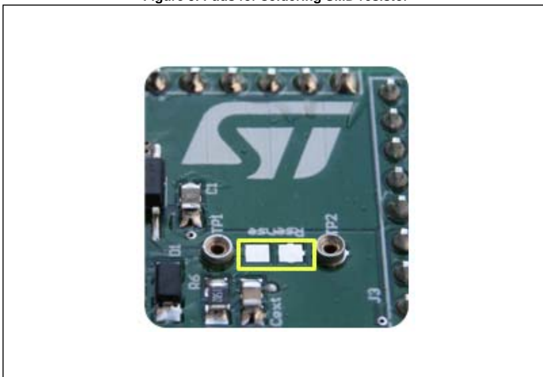
Figure 5. Pads for soldering SMD resistor
