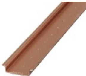
DIN rail, material: Copper, unperforated, height 7.5 mm, width 35 mm, length: 2 m
