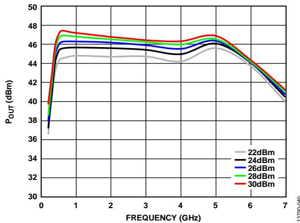
Figure 39.  $P_{OUT}$  vs. Frequency at Various Input Powers
