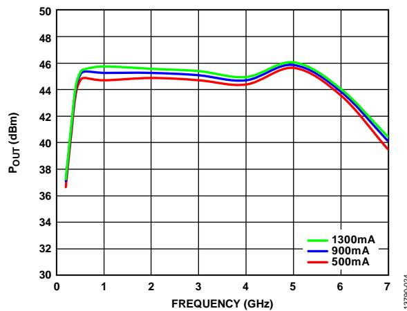
Figure 23.  $P_{OUT}$  vs. Frequency at Various Quiescent Currents ( $I_{DD1} + I_{DD2}$ ),  $P_{IN} = 24\text{ dBm}$
