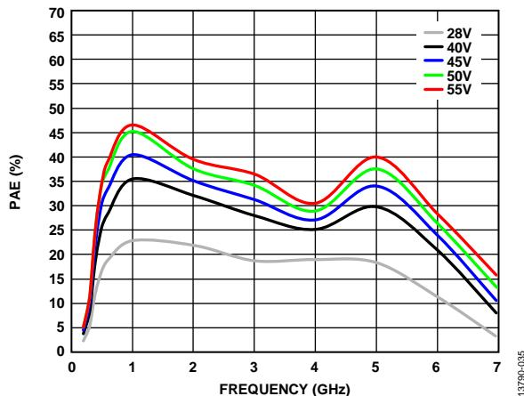
Figure 34. PAE vs. Frequency at Various Voltages,
