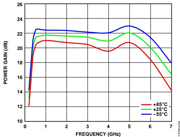
Figure 27. Power Gain vs. Frequency at Various Temperatures,
