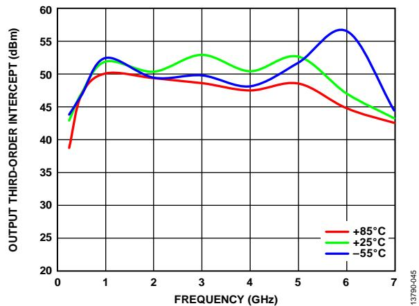
Figure 48. Output Third-Order Intercept Point (IP3) vs. Frequency at Various Temperatures,  $P_{\text{OUT}} \text{ per Tone} = 32 \text{ dBm}$
