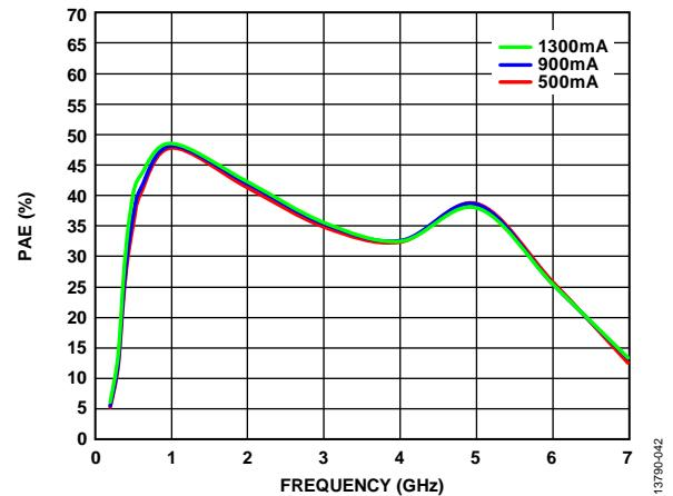
Figure 38. PAE vs. Frequency at Various Quiescent Currents ( $I_{DD1} + I_{DD2}$ ),
