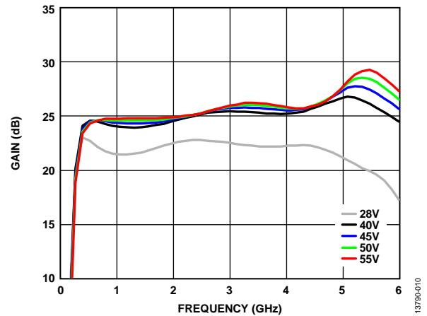
Figure 10. Gain vs. Frequency at Various Supply Voltages
