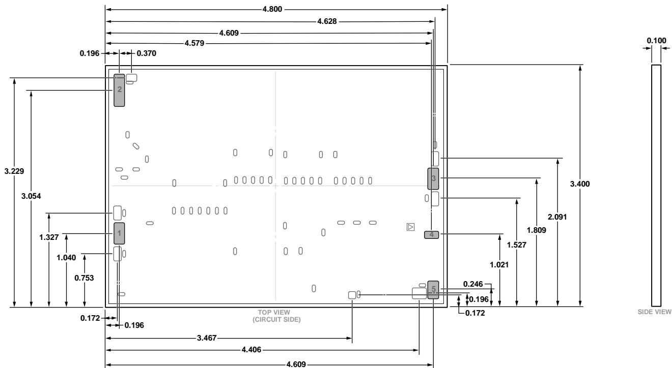
Figure 59. 5-Pad Bare Die [CHIP]
