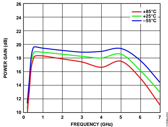
Figure 30. Power Gain vs. Frequency at Various Temperatures,
