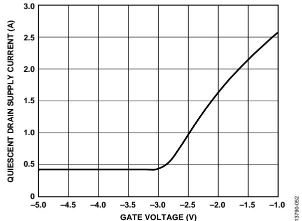
Figure 50. Quiescent Drain Supply Current vs. Gate Voltage
