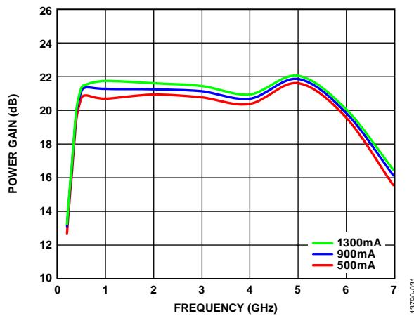
Figure 29. Power Gain vs. Frequency at Various Quiescent Currents ( $I_{DD1} + I_{DD2}$ ),
