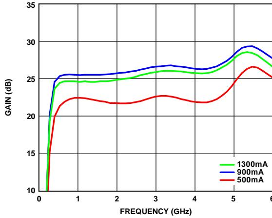
Figure 14. Gain vs. Frequency at Various Quiescent Supply Currents ( $I_{DDX}$ )
