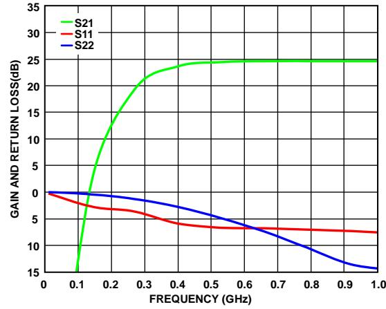
Figure 12. Gain and Return Loss vs. Frequency, 10 MHz to 1000 MHz
