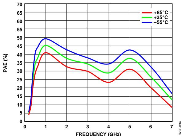
Figure 33. PAE vs. Frequency at Various Temperatures,
