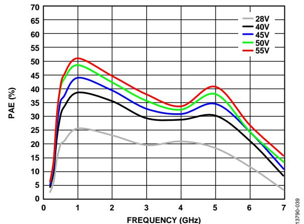
Figure 37. PAE vs. Frequency at Various Voltages,
