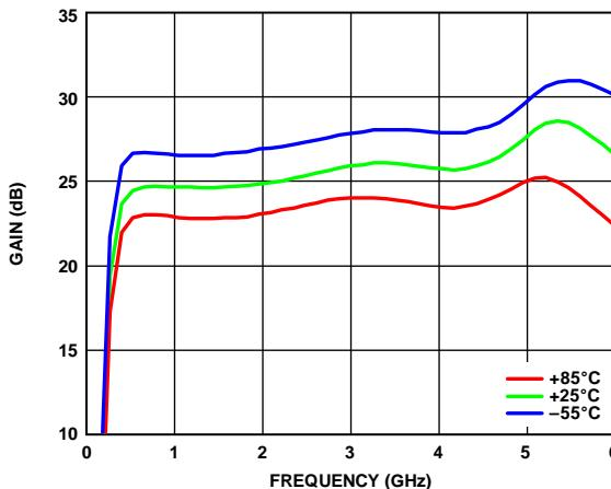
Figure 13. Gain vs. Frequency at Various Temperatures
