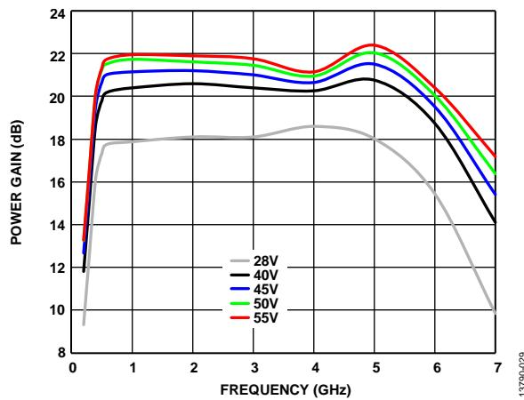
Figure 28. Power Gain vs. Frequency at Various Voltages,
