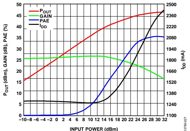
Figure 43.  $P_{OUT}$ , Gain, PAE, and Total Supply Current with RF Power Applied ( $I_{DD}$ ) vs. Input Power, Frequency = 3 GHz
