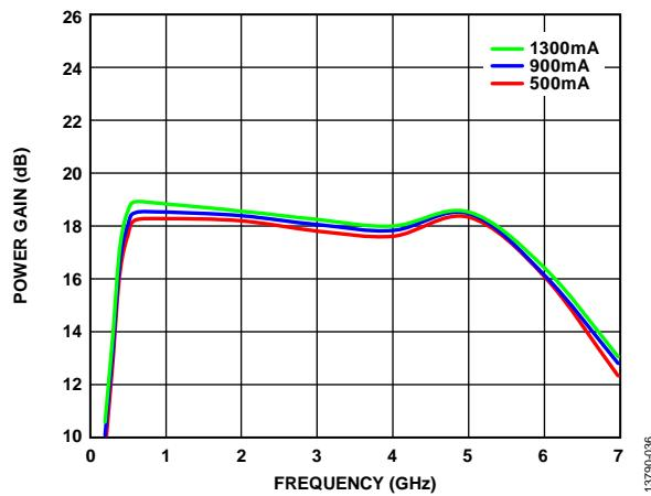
Figure 32. Power Gain vs. Frequency at Various Quiescent Currents ( $I_{DD1} + I_{DD2}$ ),
