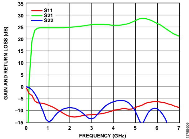
Figure 9. Gain and Return Loss vs. Frequency
