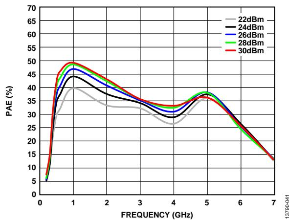
Figure 41. PAE vs. Frequency at Various Input Powers
