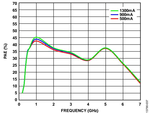
Figure 35. PAE vs. Frequency at Various Quiescent Currents ( $I_{DD1} + I_{DD2}$ ),
