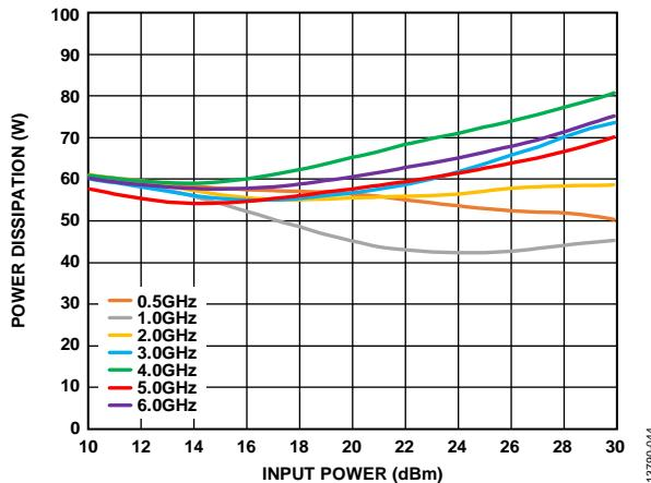
Figure 45. Power Dissipation vs. Input Power at 85°C
