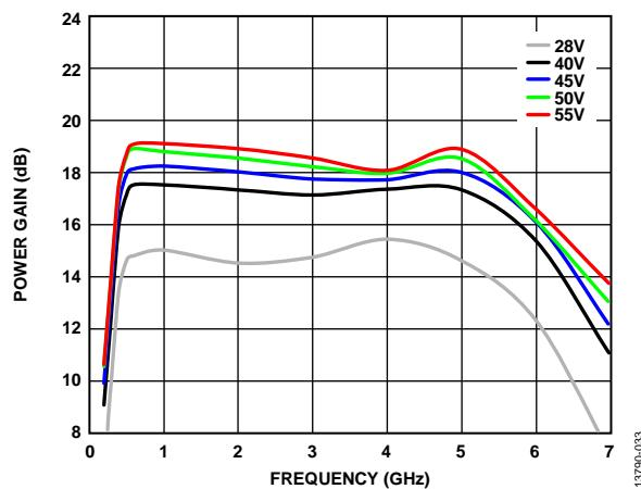
Figure 31. Power Gain vs. Frequency at Various Voltages,
