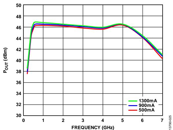
Figure 26.  $P_{OUT}$  vs. Frequency at Various Quiescent Currents ( $I_{DD1} + I_{DD2}$ ),  $P_{IN} = 28\text{ dBm}$
