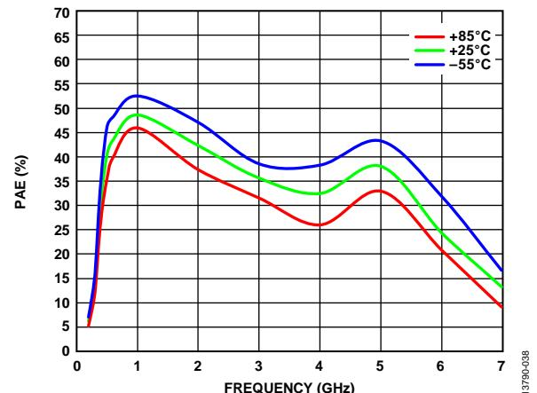
Figure 36. PAE vs. Frequency at Various Temperatures,
