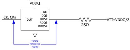
The output timing reference voltage level for single ended signals is the crosspoint with VTT. The output timing reference voltage level for differential signals is the crosspoint of the true (e.g. DQS) and the complement (e.g. DQS#) signal.
