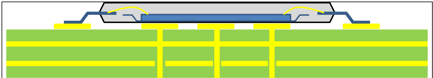
Figure 8-1: Example Thermal Via Holes on PCB.
