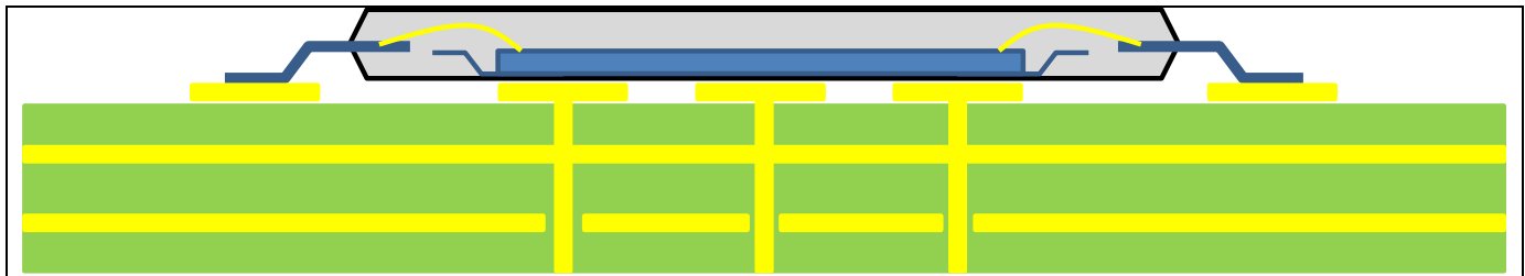
Figure 8-1: Example Thermal Via Holes on PCB.
