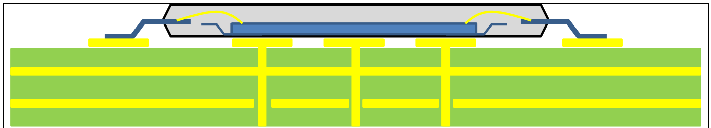
Figure 8-1: Example Thermal Via Holes on PCB.
