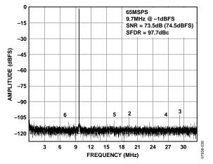
Figure 18. Single-Tone FFT with  $f_{IN} = 9.7 \text{ MHz}$
