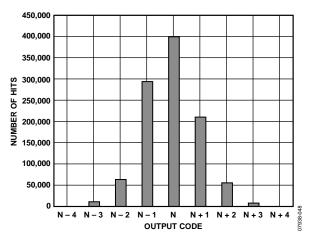
Figure 16. Grounded Input Histogram
