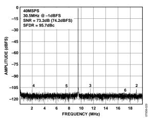
Figure 24. Single-Tone FFT with  $f_{\rm IN}$  = 30.5 MHz
