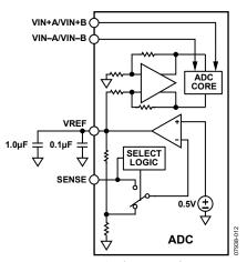
Figure 46. Internal Reference Configuration
