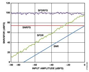
Figure 21. SNR/SFDR vs. Input Amplitude (AIN) with  $f_{\rm IN} = 9.7$  MHz
