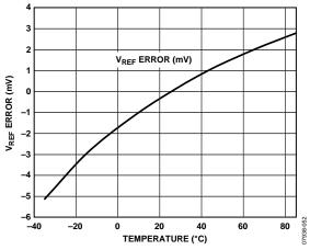
Figure 48. Typical V<sub>REF</sub> Drift
