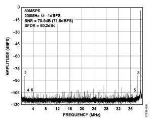
Figure 10. Single-Tone FFT with  $f_{IN} = 200 \text{ MHz}$
