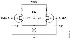
Figure 49. Equivalent Clock Input Circuit
