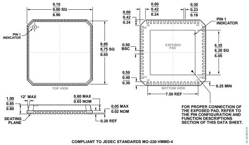
Figure 59. 64-Lead Lead Frame Chip Scale Package [LFCSP\_VQ] 9 mm × 9 mm Body, Very Thin Quad (CP-64-4) Dimensions shown in millimeters
