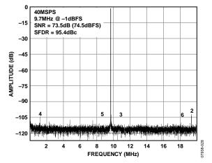
Figure 23. Single-Tone FFT with  $f_{\rm IN}$  = 9.7 MHz
