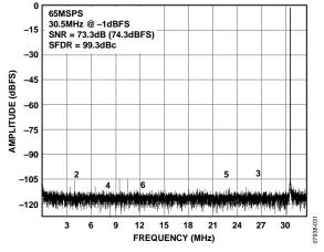
Figure 20. Single-Tone FFT with  $f_{IN} = 30.5$  MHz
