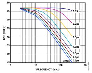
Figure 56. SNR vs. Input Frequency and Jitter
