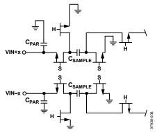
Figure 38. Switched-Capacitor Input Circuit
