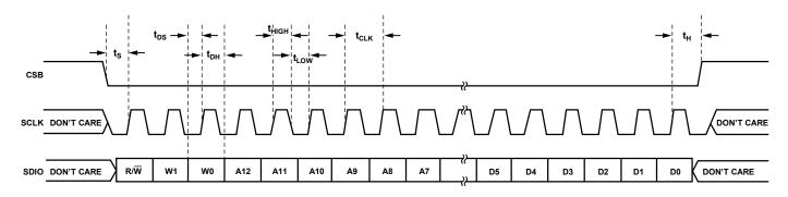
Figure 58. Serial Port Interface Timing Diagram
