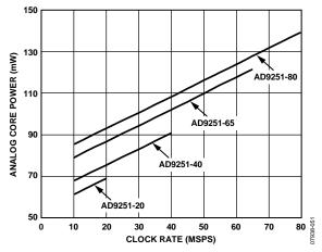
Figure 57. Analog Core Power vs. Clock Rate
