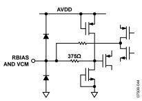
Figure 34. Equivalent RBIAS, VCM Circuit
