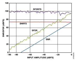
Figure 15. SNR/SFDR vs. Input Amplitude (AIN) with  $f_{\text{IN}} = 9.7 \text{ MHz}$
