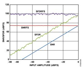
Figure 25. SNR/SFDR vs. Input Amplitude (AIN) with  $f_{\rm IN} = 9.7$  MHz
