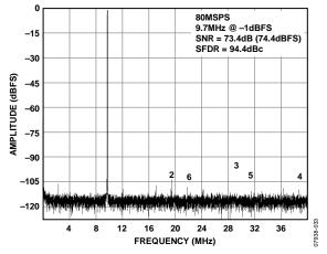
Figure 6. Single-Tone FFT with  $f_{IN} = 9.7 \text{ MHz}$
