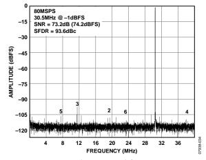
Figure 9. Single-Tone FFT with  $f_{IN} = 30.5$  MHz
