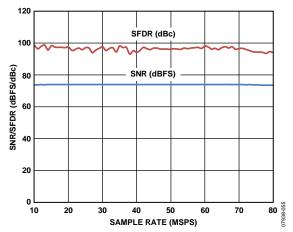
Figure 13. SNR/SFDR vs. Sample Rate with AIN = 9.7 MHz
