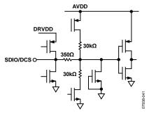
Figure 31. Equivalent SDIO/DCS Input Circuit
