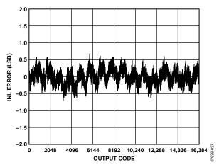
Figure 17. INL with  $f_{IN} = 9.7 \text{ MHz}$
