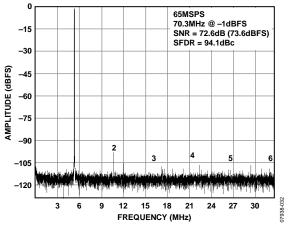
Figure 19. Single-Tone FFT with  $f_{IN} = 70.3$  MHz
