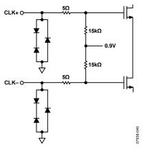
Figure 30. Equivalent Clock Input Circuit
