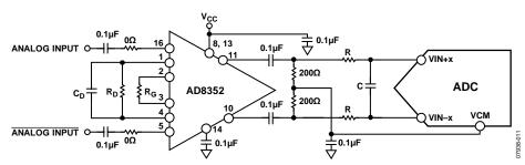
Figure 45. Differential Input Configuration Using the AD8352
