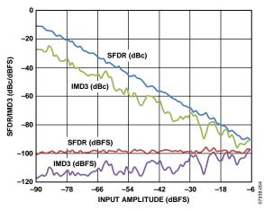
Figure 11. Two-Tone SFDR/IMD3 vs. Input Amplitude (AIN) with  $f_{\rm IN1} = 30.5$  MHz and  $f_{\rm IN2} = 32.5$  MHz
