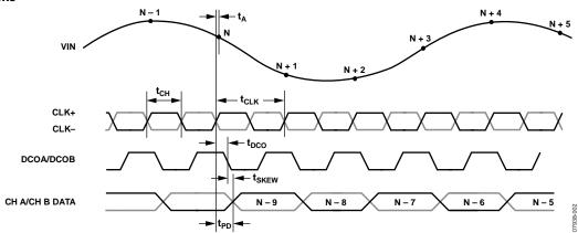
Figure 2. CMOS Output Data Timing
