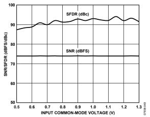
Figure 39. SNR/SFDR vs. Input Common-Mode Voltage,  $f_{\rm IN} = 32.1$  MHz,  $f_{\rm S} = 80$  MSPS
