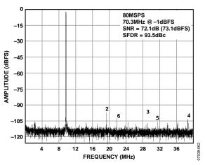
Figure 7. Single-Tone FFT with  $f_{IN} = 70.3 \text{ MHz}$
