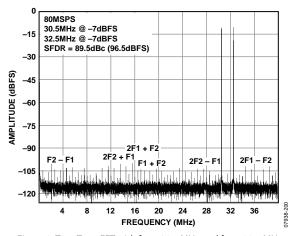
Figure 8. Two-Tone FFT with  $f_{\text{IN1}} = 30.5$  MHz and  $f_{\text{IN2}} = 32.5$  MHz
