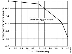
Figure 47. VREF Accuracy vs. Load Current
