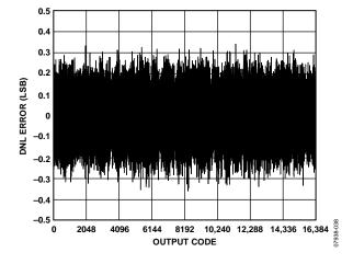
Figure 14. DNL Error with  $f_{\text{IN}} = 9.7 \, \text{MHz}$
