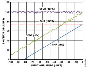
Figure 28. SNR/SFDR vs. Input Amplitude (AIN) with  $f_{\rm IN} = 9.7$  MHz
