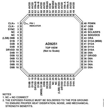
Figure 5. Pin Configuration
