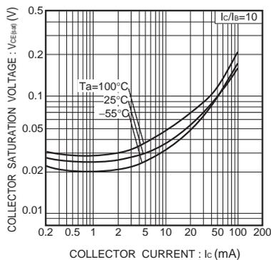
Fig.7 Collector-emitter saturation voltage vs. collector current ( I )
