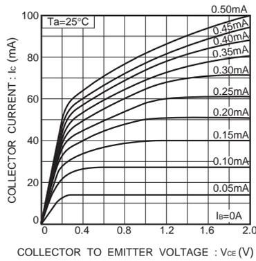
Fig.2 Grounded emitter output characteristics ( I )
