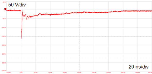
Figure 5. ESD response to ISO 10605 - C = 150 pF, R = 330 \Omega (-8 kV contact discharge)
