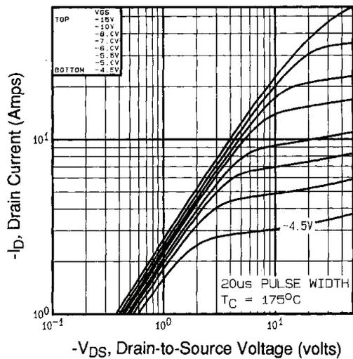
Fig. 2 - Typical Output Characteristics,  $T_C = 175^\circ\text{C}$
