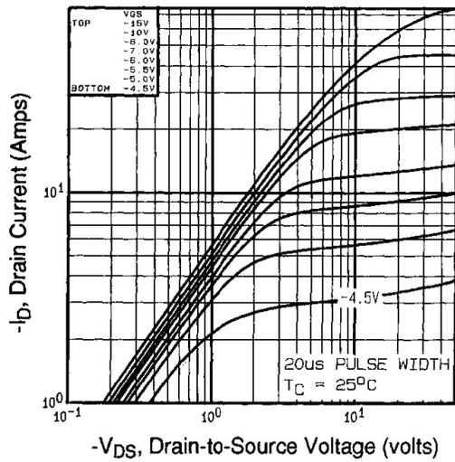
Fig. 1 - Typical Output Characteristics,  $T_C = 25^\circ\text{C}$
