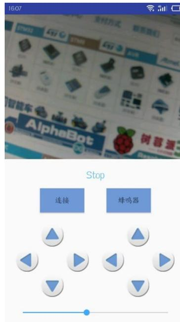
Enter the actual IP address of RPi, and click the button **Connect**. Then, you can see the images captured by the camera. Next, click the button **Connect** under the image. When the control port has been connected to the program, this button will change from green to blue. Now, you can control the actions of the smart robot and the steer by pressing down the corresponding keys. By dragging the slider, you can change the speed of the robot.
