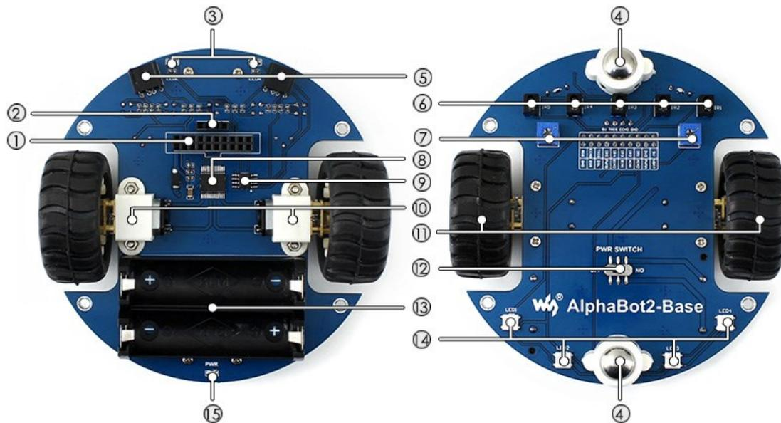
1. **AlphaBot2 control interface:** for connecting sorts of controller adapter board
