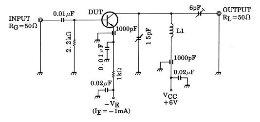
L1: 0.8 mm $\phi$  silver plated copper wire, 4 T, 10 mm ID, 8 mm length
