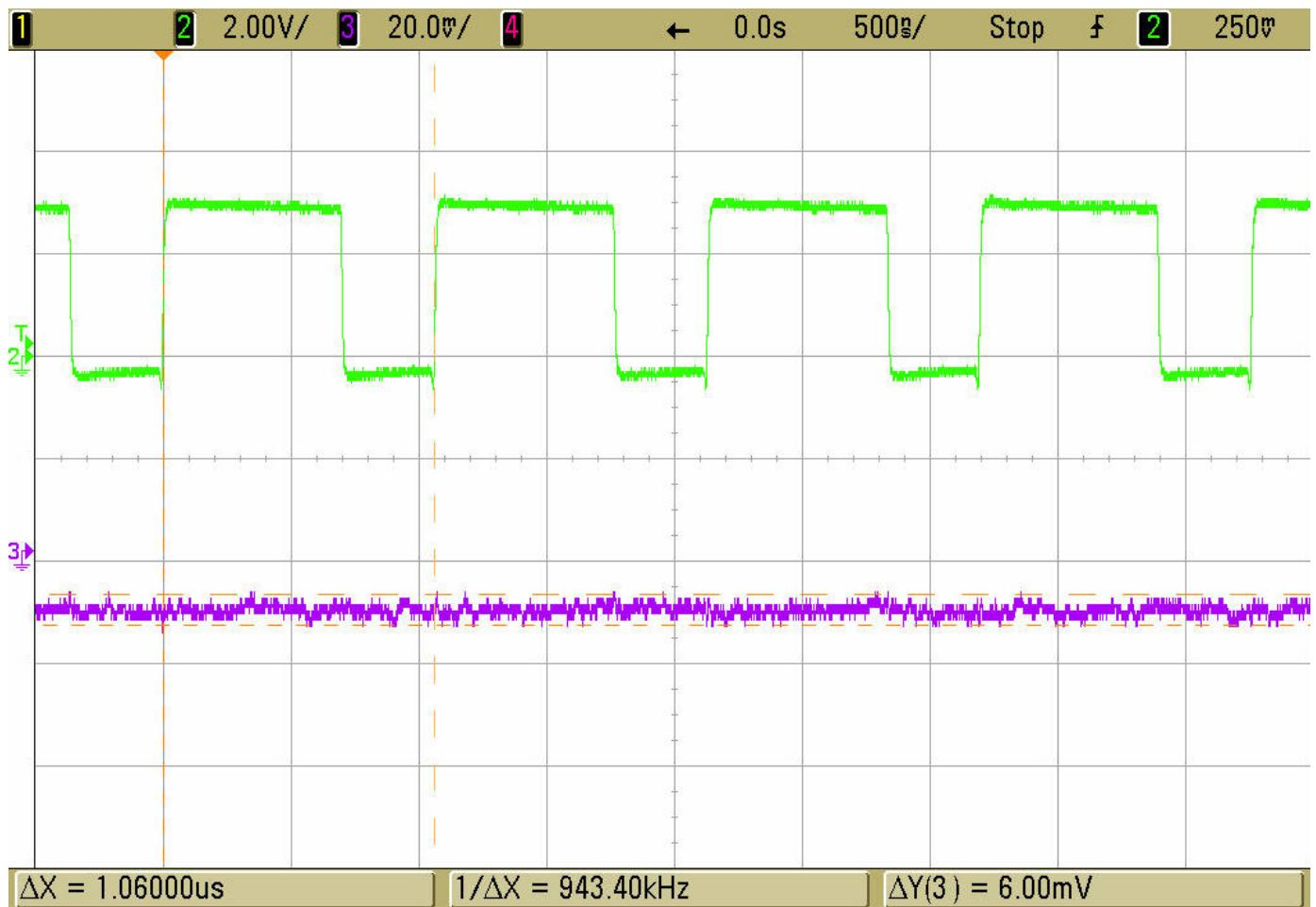
**Figure 3. Switch Waveform & Output Ripple Voltage**
