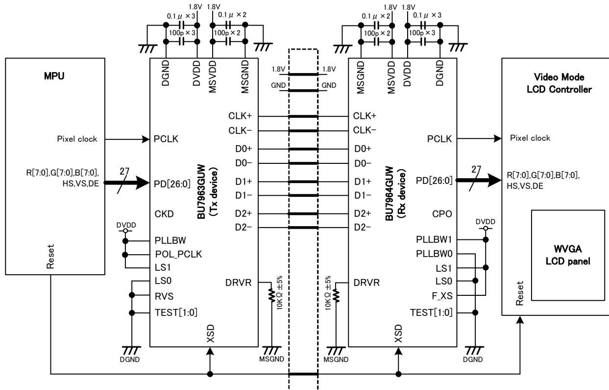
Fig.15. Application Circuit
