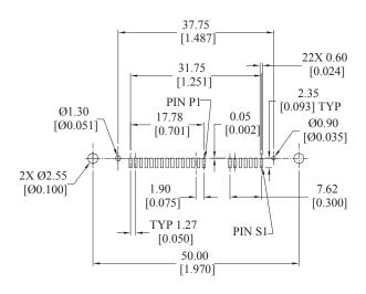
RECOMMENDED PCB LAYOUT TOLERANCE:  $\pm 0.05 [0.002]$
