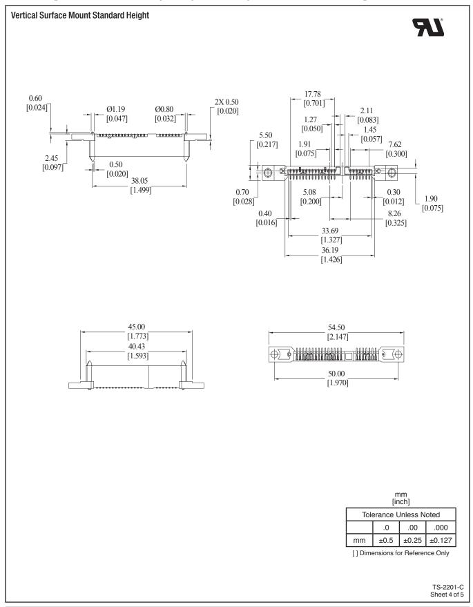
Host Receptacle, Vertical and Right Angle, Std Height, Surface Mount Receptacle 5622 Series
