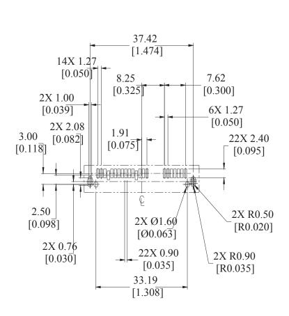
RECOMMENDED P.C.B. LAYOUT TOLERANCE : ± 0.05 [.002] TOP VIEW
