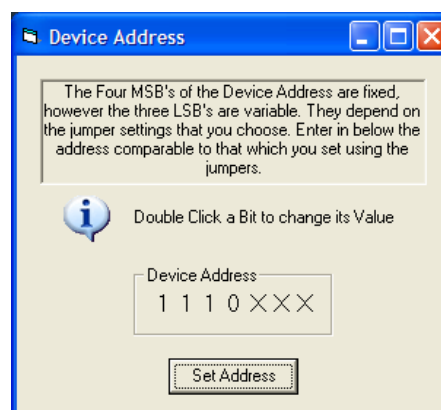
Figure 3. I 2 C Address Selection
