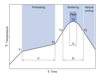
Preheating Soldering Peak Temp. Time Temp. Time Temp. Time T1 T2 Т3 **T4** t3 150°C 180°C 60 to 120s 230°C 30s 260°C 10s
