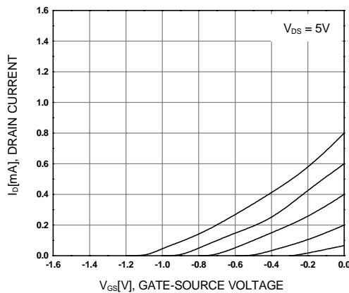
**Figure 3.  $I_D$ - $V_{GS}$**
