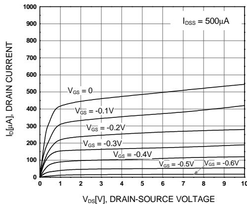
**Figure 2.  $I_D$ - $V_{DS}$**
