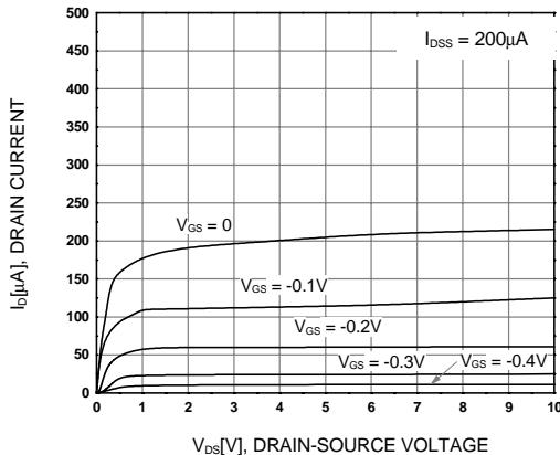
**Figure 1.  $I_D$ - $V_{DS}$**
