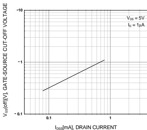
**Figure 5.  $V_{GS(\text{off})}$ - $I_{DSS}$**
