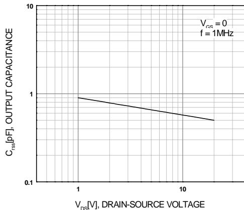
Figure 7.  $C_{RSS}$ - $V_{DS}$
