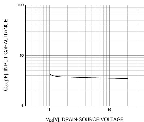
**Figure 6.  $C_{iss}$ - $V_{DS}$**
