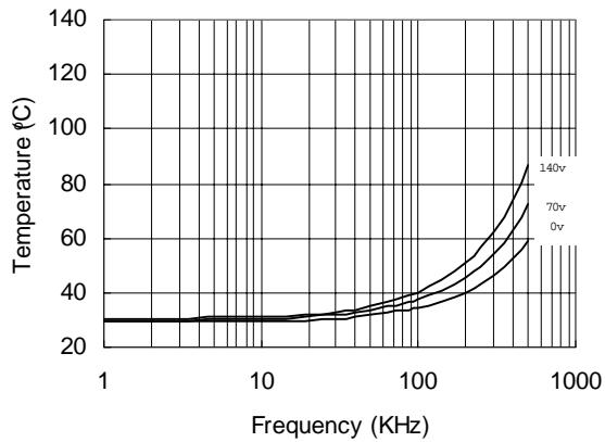
Figure 23. IR2183 vs. Frequency (IRFBC30),
