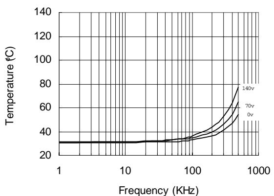
Figure 30. IR2183s vs. Frequency (IRFBC20),
