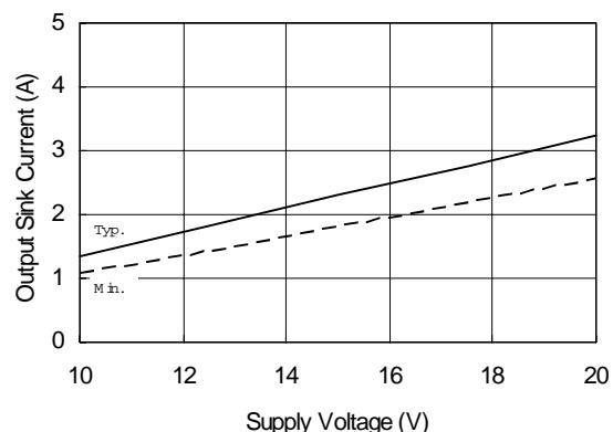
**Figure 21B. Output Sink Current vs. Supply Voltage**
