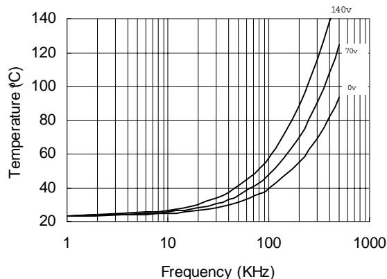
Figure 29. IR21834 vs. Frequency (IRFPE50),
