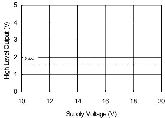
**Figure 11B. High Level Output vs. Supply Voltage**
