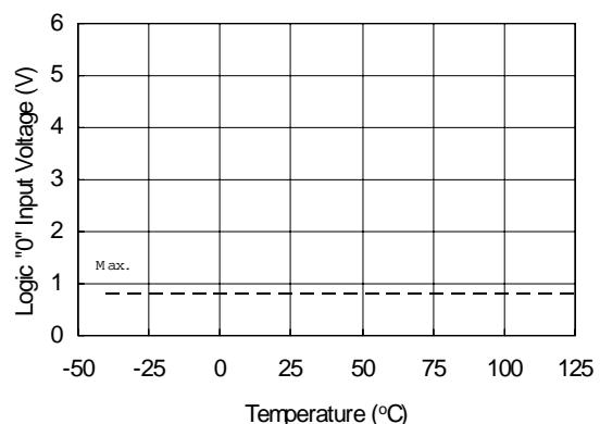
**Figure 10A. Logic "0" Input Voltage vs. Temperature**
