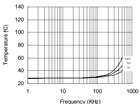
Figure 34. IR21834s vs. Frequency (IRFBC20),
