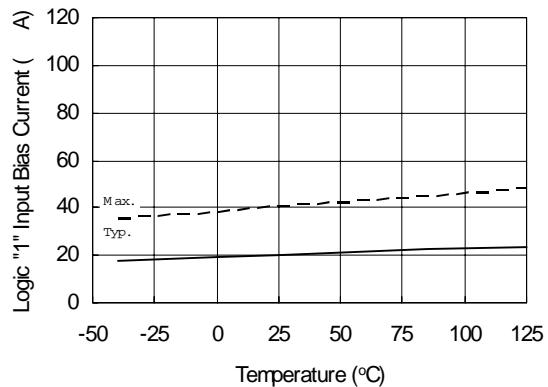
**Figure 16A. Logic "1" Input Bias Current vs. Temperature**
