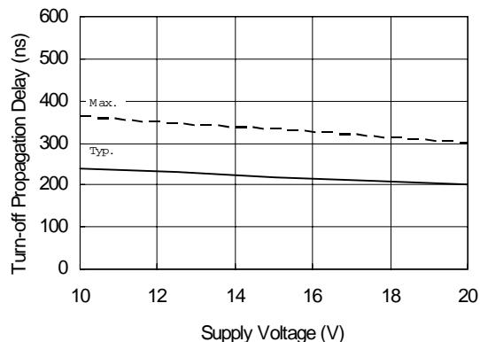
**Figure 5B. Turn-off Propagation Delay vs. Supply Voltage**
