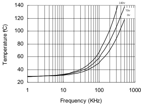
Figure 25. IR2183 vs. Frequency (IRFPE50),
