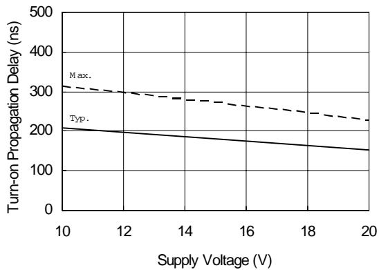
**Figure 4B. Turn-on Propagation Delay vs. Supply Voltage**
