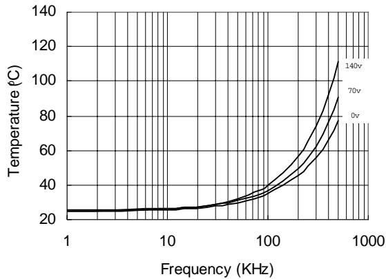
Figure 31. IR2183s vs. Frequency (IRFBC30),
