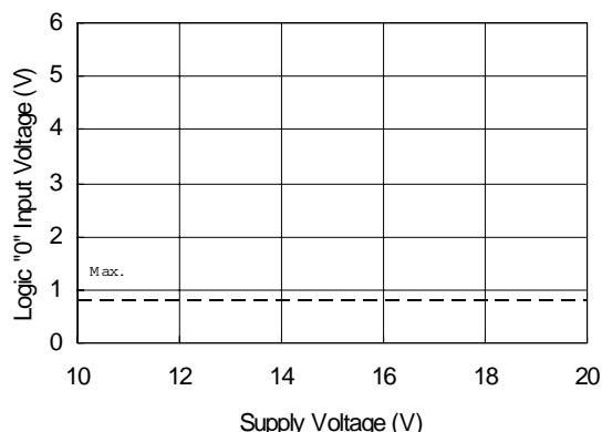
**Figure 10B. Logic "0" Input Voltage vs. Supply Voltage**
