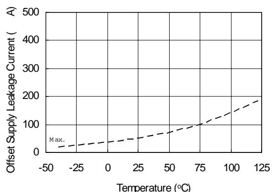
**Figure 13A. Offset Supply Leakage Current vs. Temperature**
