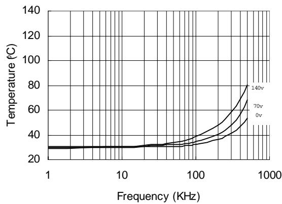
Figure 35. IR21834s vs. Frequency (IRFBC30),
