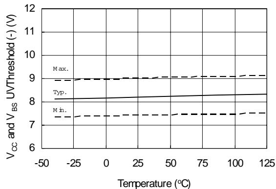
**Figure 19.  $V_{CC}$  and  $V_{BS}$  Undervoltage Threshold (-) vs. Temperature**
