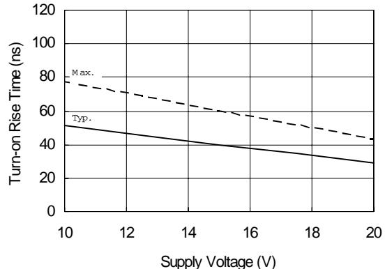
Figure 6B. Turn-on Rise Time vs. Supply Voltage
