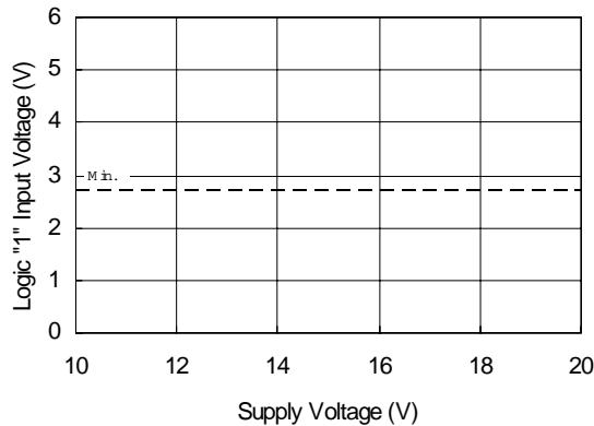
**Figure 9B. Logic "1" Input Voltage vs. Supply Voltage**
