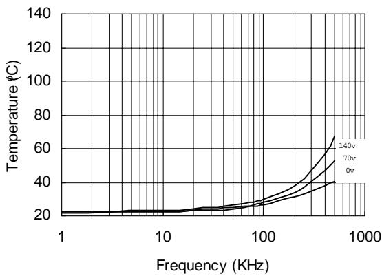
Figure 27. IR21834 vs. Frequency (IRFBC30),
