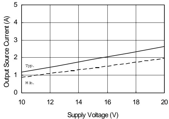
**Figure 20B. Output Source Current vs. Supply Voltage**
