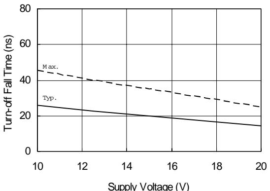
Figure 7B. Turn-off Fall Time vs. Supply Voltage
