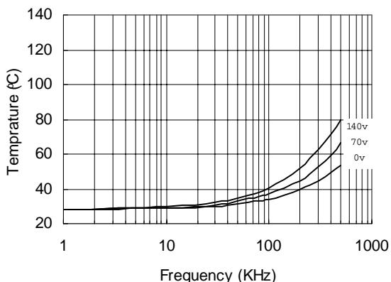
**Figure 22. IR2183 vs. Frequency (IRFBC20),
