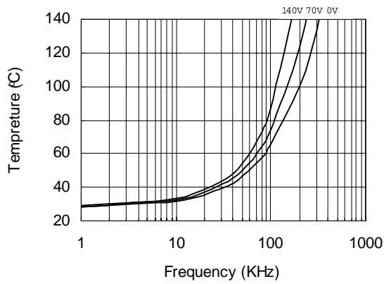
Figure 33. IR2183s vs. Frequency (IRFPE50),
