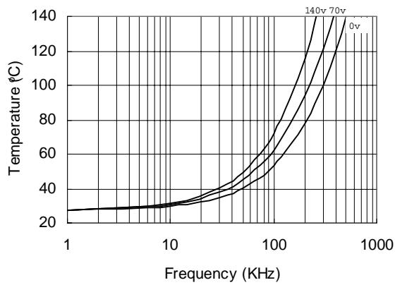
Figure 37. IR21834s vs. Frequency (IRFPE50),
