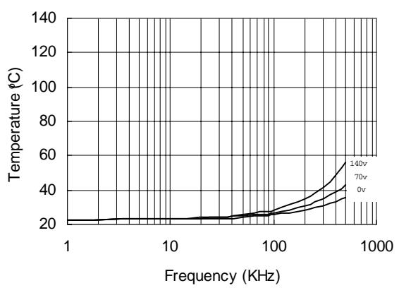
Figure 26. IR21834 vs. Frequency (IRFBC20),
