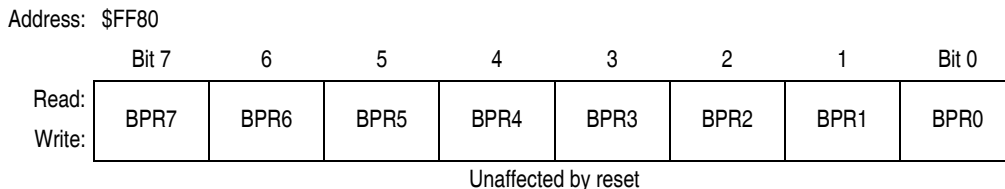
Figure 2-4. FLASH-1 Block Protect Register (FL1BPR)
