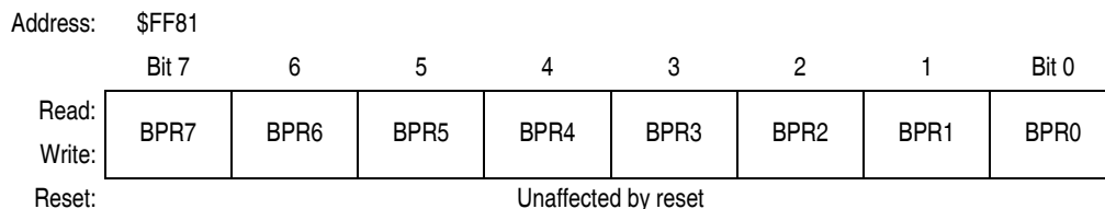
Figure 2-8. FLASH-2 Block Protect Register (FL2BPR)
