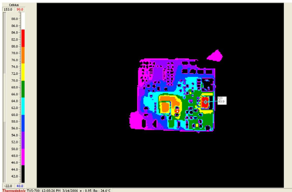
Figure 8. Temp Data (48Vin, 8A, 100LFM airflow – back)
