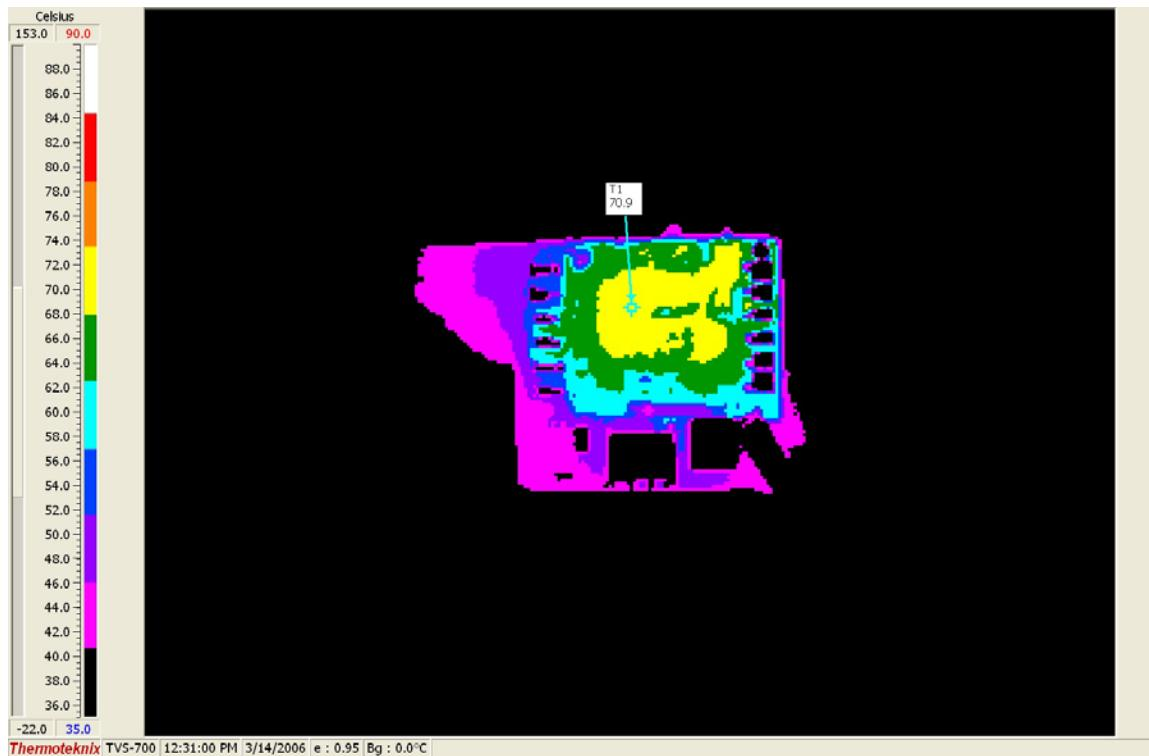
Figure 7. Temp Data (48Vin, 5A, 100LFM airflow – front)
