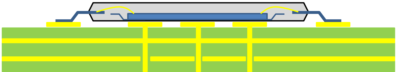
Figure 10.2-1: Example thermal via holes on PCB.
