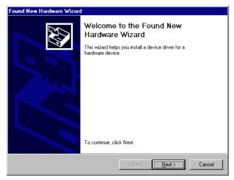
The wizard will ask you to help determine the correct driver files for the new device. First select the **Search for a suitable driver for my device (recommended)** option, then click the **Next** button.
