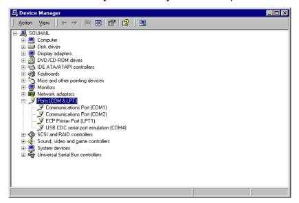
You should see the **USB CDC serial port emulation (COM**x), where x gives the COM port number has Windows has assigned to the device.
