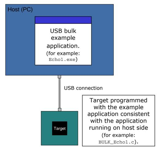
To use this application, make sure to use the corresponding example files both on the host-side as on the target side. The example applications on the PC host are named in the same way, just without the prefix BULK\_, for example, if the host runs Echol.exe, BULK\_Echol.c has to be included into your project, compiled and downloaded into your target. There are additional examples that can be used for testing emUSB.
