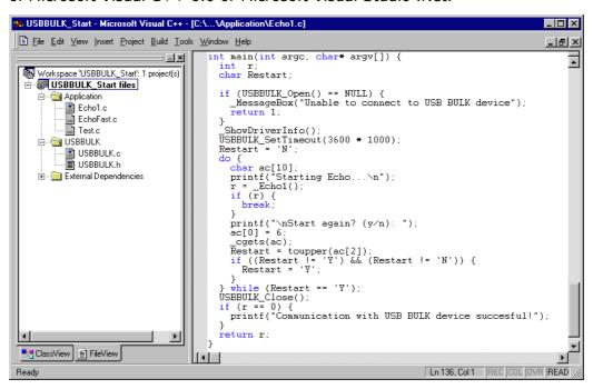
The source code of the sample application is located in the subfolder Bulk\SAMPLEAPP. Open the file USBBULK\_Start.dsw and compile the source choose **Build | Build SampleApp.exe** (Shortcut: F7). To run the executable choose **Build | Execute SampleApp.exe** (Shortcut: CTRL-F5).
