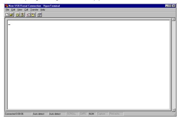
Type any characters, these characters will be sent to target. The echo of the target is shown in the terminal window:
