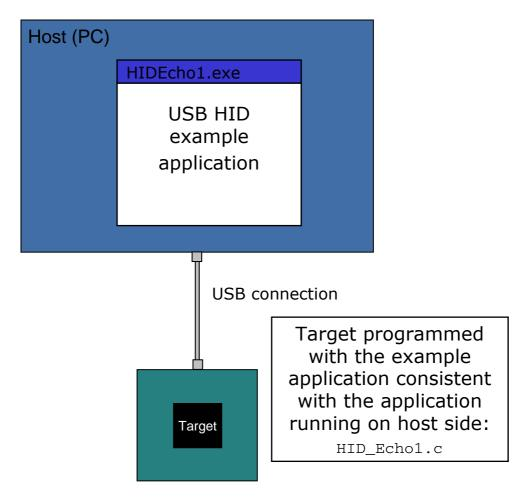
To use this application, include the source code file HID\_Echo1.c into your project and compile and download it into your target. Run HIDEcho1.exe after the target is connected to the host and the enumeration process has been completed. The PC application is supplied as executable in the HID\SampleApp\Exe directory. The source code of the PC example is also supplied. Refer to section *Compiling the PC example application* on page 343 for more information to the PC example project.
