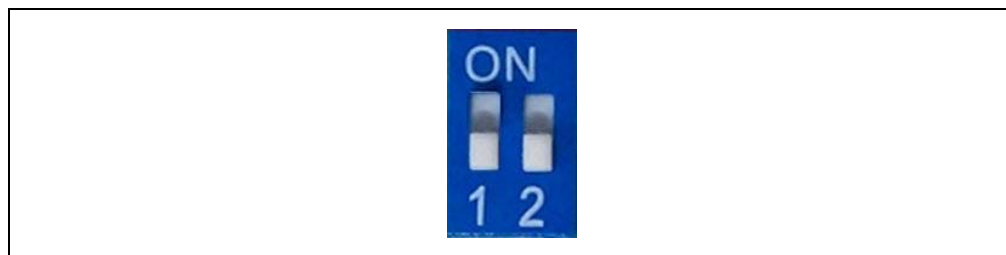
FIGURE 3-35: SWITCH SW9 IN FLASH APPLICATION MODE
