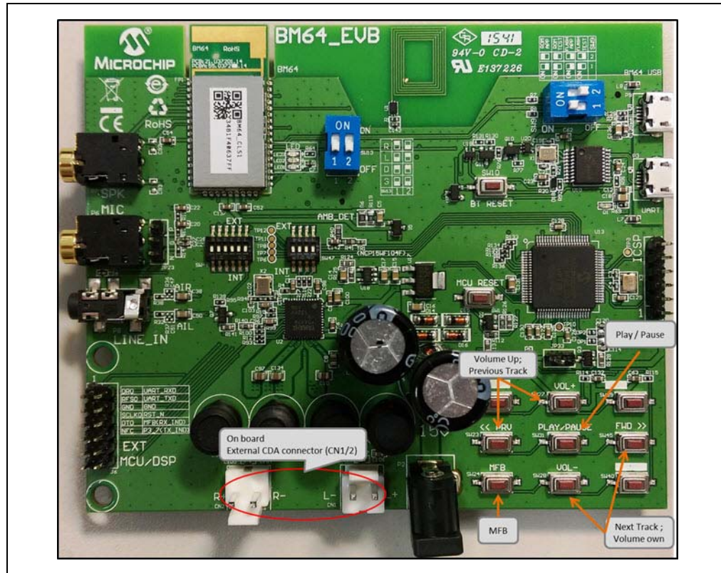
FIGURE 3-4: BM64 EVB AUDIO CONTROL BUTTONS
