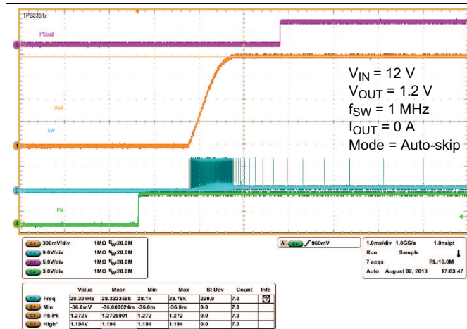
Figure 19. Auto-Skip Mode Load Transient
