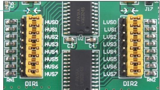
**Figure 5:** Jumpers DIR1 and DIR2 in the position for 3.3V to 5V voltage level adjustment
