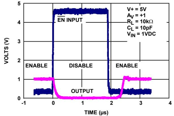
FIGURE 16. ENABLE/DISABLE TIMING
