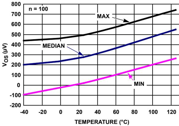
FIGURE 21.  $V_{OS}$  vs TEMPERATURE,  $V_S = \pm 2.5V$
