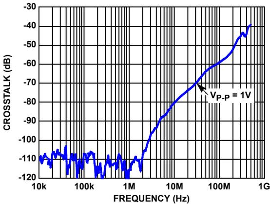
FIGURE 11. CHANNEL TO CHANNEL CROSSTALK vs FREQUENCY
