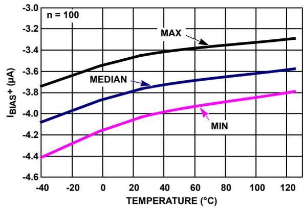
FIGURE 22.  $I_{BIAS+}$  vs TEMPERATURE,  $V_S = \pm 2.5V$
