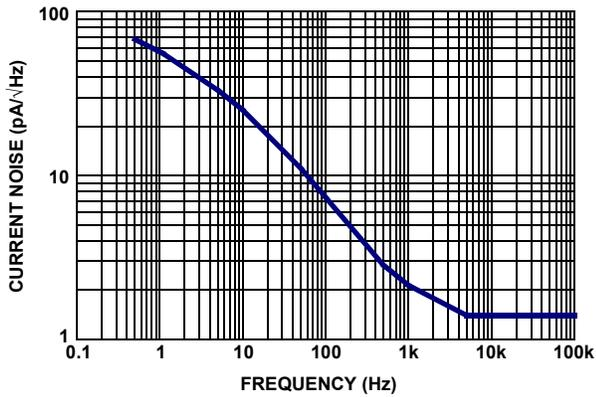
FIGURE 15. INPUT REFERRED NOISE CURRENT vs FREQUENCY
