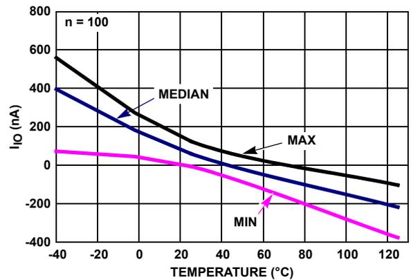
FIGURE 24.  $I_{IO}$  vs TEMPERATURE,  $V_S = \pm 2.5V$
