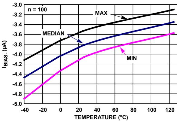
FIGURE 23.  $I_{BIAS-}$  vs TEMPERATURE,  $V_S = \pm 2.5V$
