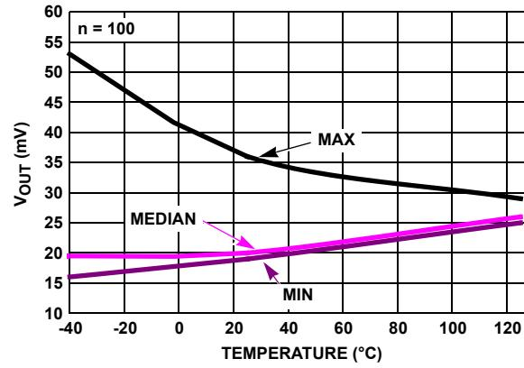
FIGURE 28. NEGATIVE  $V_{OUT}$  vs TEMPERATURE,  $R_L = 1k$
