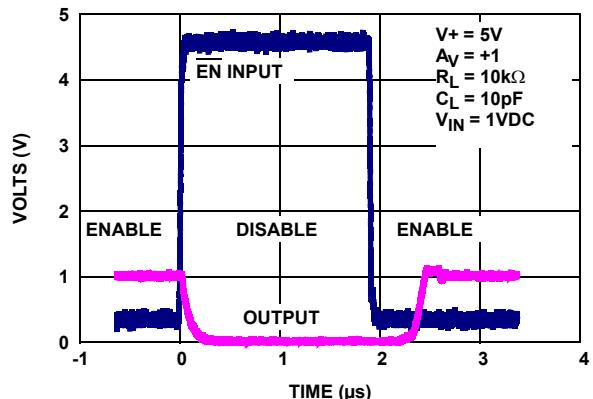
FIGURE 16. ENABLE/DISABLE TIMING
