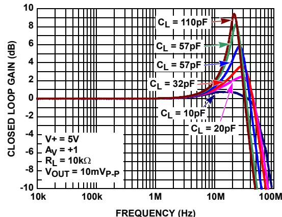
FIGURE 2. GAIN vs FREQUENCY FOR VARIOUS  $C_{LOAD}$
