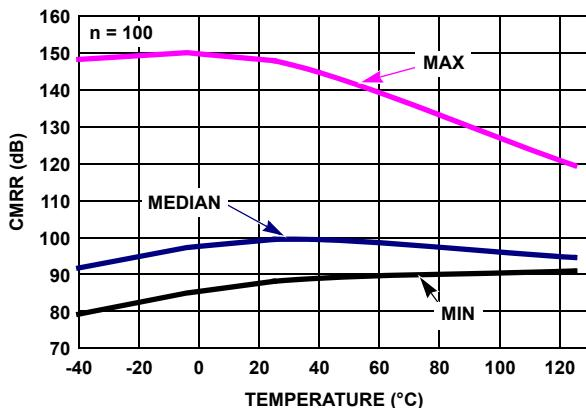
FIGURE 25. CMRR vs TEMPERATURE,  $V_{CM} = 3.8V$ ,
