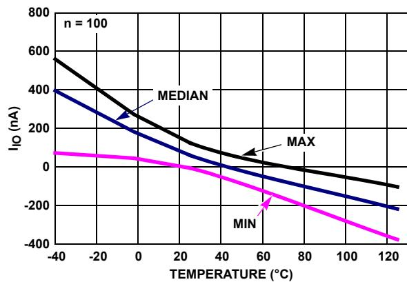
FIGURE 24.  $I_O$  vs TEMPERATURE,  $V_S = \pm 2.5V$
