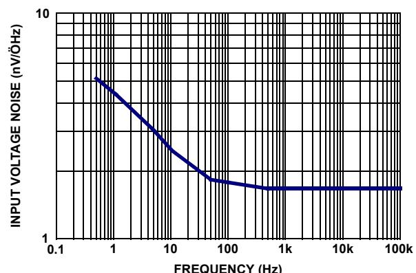
FIGURE 14. INPUT REFERRED NOISE VOLTAGE vs FREQUENCY
