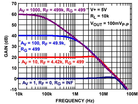
FIGURE 4. FREQUENCY RESPONSE vs CLOSED LOOP GAIN
