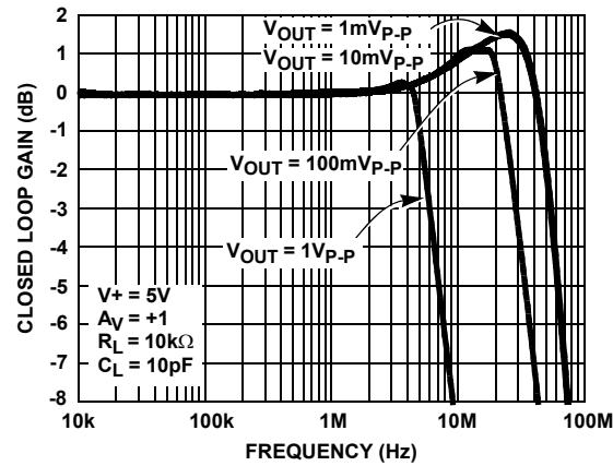
FIGURE 3. -3dB BANDWIDTH vs  $V_{OUT}$
