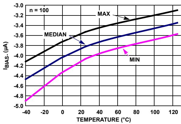
FIGURE 23.  $I_{BIAS-}$  vs TEMPERATURE,  $V_S = \pm 2.5V$
